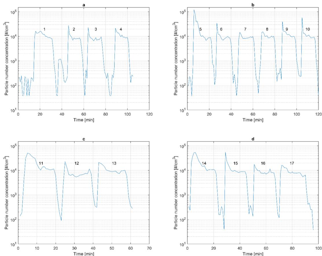
Fig. 4 Particle number concentration as measured by the MiniWRAS®. Note the logarithmic scale on the ordinate. (a) First day, with tests 1–4, (b) second day, with tests 5–10, (c) third day, with tests 11–13, and (d) fourth day, with tests 14–17.
