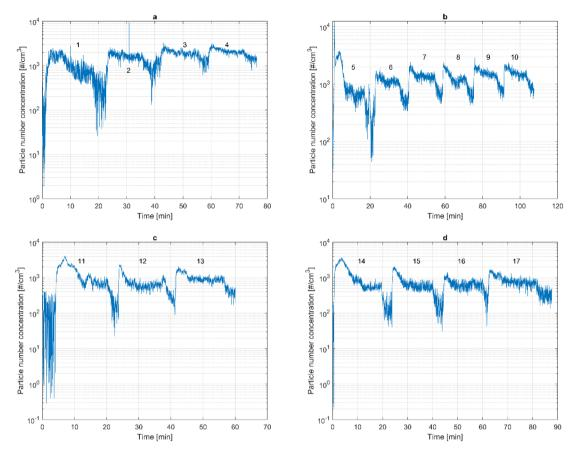
Particle number concentration as measured by the ELPI+. Note the logarithmic scale on the ordinate. (a) First day, with tests 1-4, (b) second day, with tests 5-10, (c) third day, with tests 11-13, and (d) fourth day, with tests 14-17.
