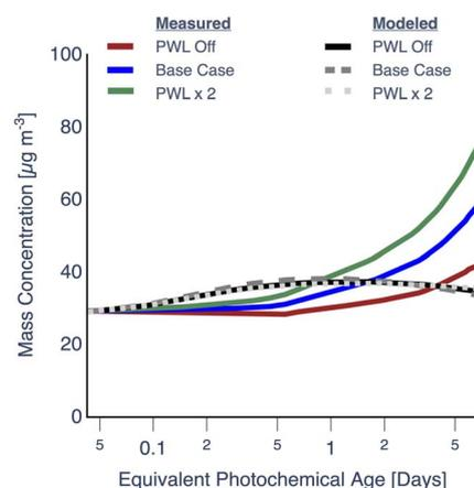
Fig. 2 SOM-TOMAS model predictions and measurements for OA mass concentrations assuming no particle wall losses (PWL off),  $\tau_{\text{PWL}} = 72 \text{ min}$  (Base), and  $\tau_{\text{PWL}} = 36 \text{ min}$  (PWL  $\times 2$ ) for the ponderosa pine chamber experiment (Fire 38). The modeled and measured OA mass concentrations have been corrected for dilution and PWL.
