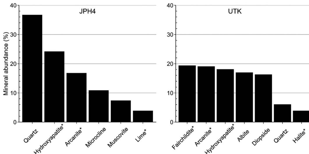
Fig. 5 Mineral abundance (%) from XRD analyses of *Sphagnum* moss ash samples collected from JPH4 and UTK in October 2020. UTK = Utikuma. The asterisks (\*) indicate minerals created during ashing. Note: Ignoring the minerals created during ashing, quartz accounts for 66.7% of the ash at JPH4 and 15.5% of the ash at UTK.
