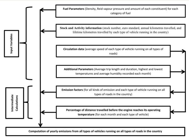
Fig. 1 Application of the fundamental methodology of COPERT.<sup>15</sup>
