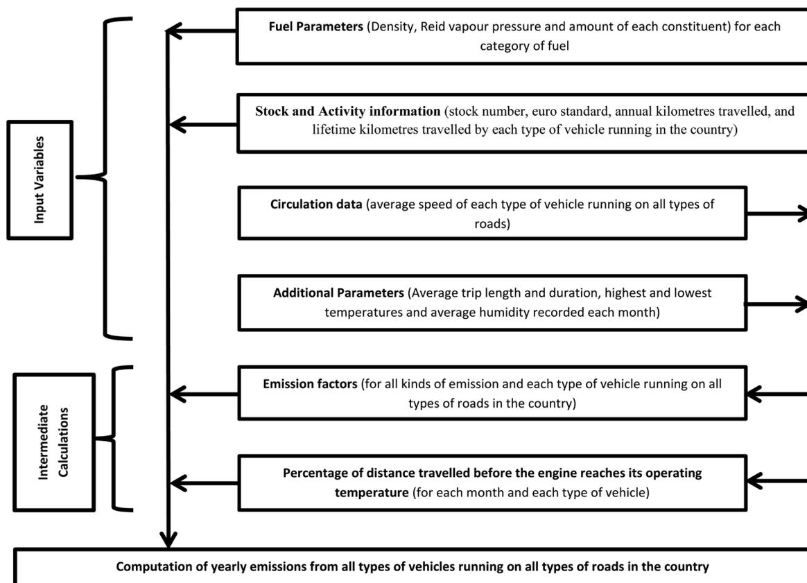
Fig. 1 Application of the fundamental methodology of COPERT.<sup>15</sup>
