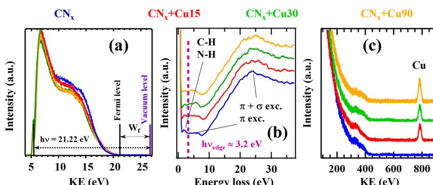
Fig. 5 (a) UPS work function determination for the indicated specimens ( $W_f$  = work function); (b) REELS spectra showing the presence of the  $\pi$  and  $\pi + \sigma$  plasmonic excitation typical of such composite materials. The incorporation of H atoms is evidenced by the small peak centred at  $\approx 2$  eV, while the optical band gap is estimated at  $\approx 3.2$  eV. (c) ISS spectra highlighting the different Cu<sub>x</sub>O surface contents for the composite samples.
