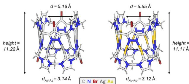
**Fig. 2** Molecular structures of the cations of  $\text{Ag}_8(\text{L}^{\text{Br}2})_2(\text{PF}_6)_4$  and  $\text{Au}_8(\text{L}^{\text{Br}2})_2(\text{PF}_6)_4$ . Counterions, solvent molecules and disorders are omitted for clarity. The distance  $d$  corresponds to the pore opening as defined in the ESI.†
