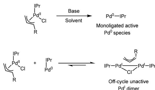
Fig. 2 Scheme of the activation and the dimerization *via* comproportionation presented by the Hazari group.<sup>49</sup>
