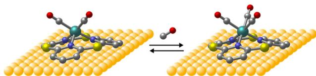
**Fig. 1** Concept of a hybrid catalytic system by deposition dome-shaped metal–organic complexes (MOCs) on metal surfaces providing the opportunity to bind and catalytically convert molecules from the gas phase. (Shown are DFT optimized gas phase structures positioned on a surface).
