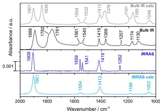
**Fig. 4** Calculated and measured vibrational spectra of [Mo(CO)<sub>3</sub>(Py<sub>3</sub>S<sub>3</sub>)] (1) in bulk material and adsorbed on Au(111) surfaces.
