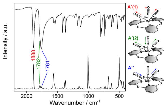
**Fig. 3** IR (top) and Raman (bottom) spectra of [Mo(CO)<sub>3</sub>(Py<sub>3</sub>S<sub>3</sub>)] (1) between 2200 cm<sup>-1</sup> and 400 cm<sup>-1</sup>. The Raman data were multiplied with the factor of 30.
