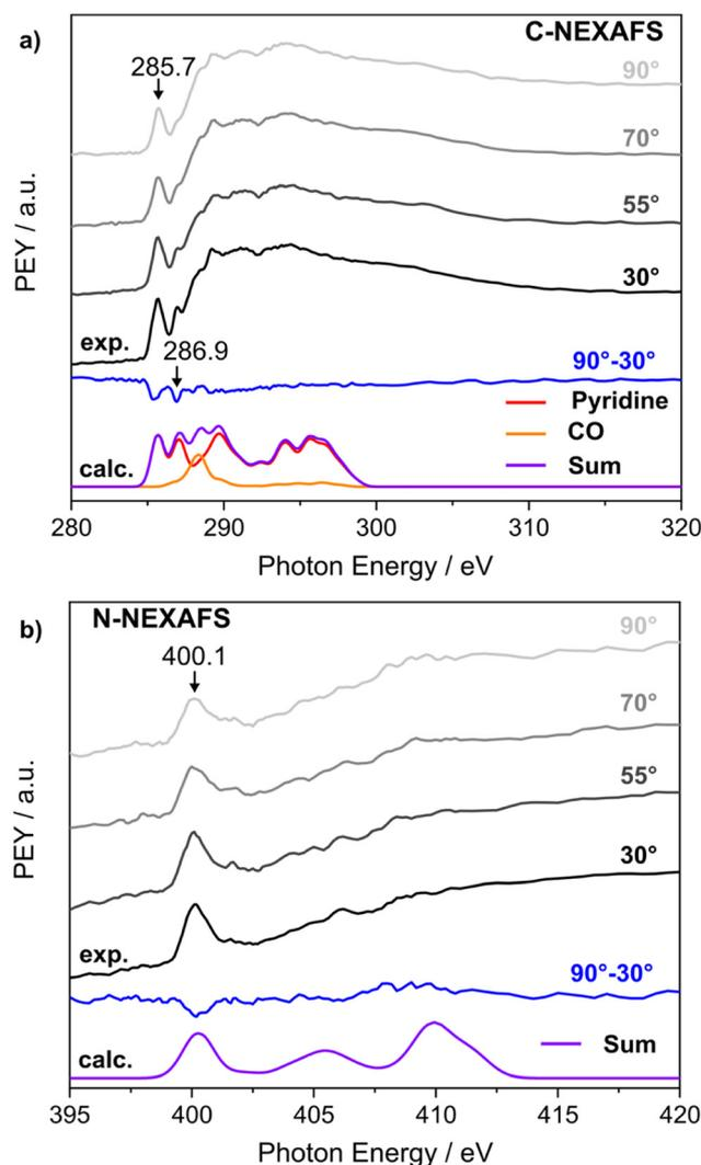
Fig. 7 Normalized NEXAFS spectra of a monolayer of [Mo(CO)<sub>3</sub>(Py<sub>3</sub>S<sub>3</sub>)] (**1**) on Au(111) at different angles (30°, 55°, 70°, 90°) and the calculated NEXAFS data (shifted by +11.4 eV (C) and +13.3 eV (N)) with the contribution of the different subunits summed over all angles: (a) C K-edge spectrum; (b) N K-edge spectrum.
