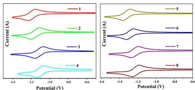
Fig. 4 Cyclic voltammogram of boron complexes 1–8 at a scan rate of  $50 \text{ mV s}^{-1}$  in dichloromethane (0.1 M of  ${}^n\text{Bu}_4\text{N}[\text{PF}_6]$  as the supporting electrolyte, vs.  $\text{Fc}/\text{Fc}^+$ ).
