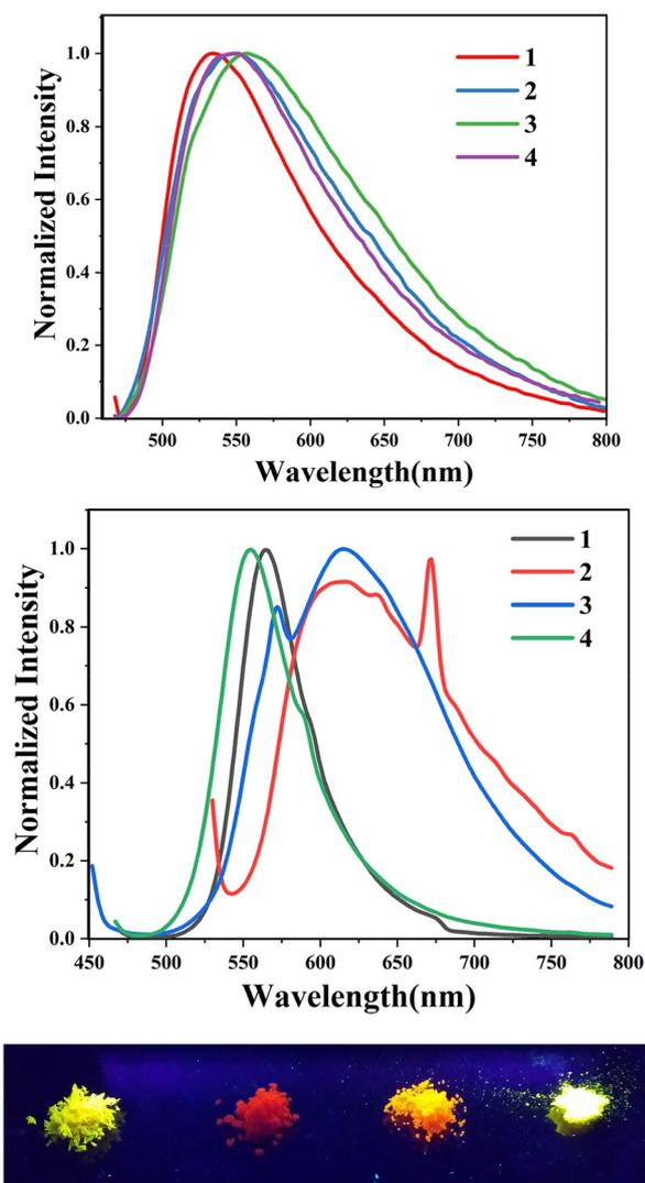
Fig. 3 (top) Photoluminescence spectra of complexes 1–4 ( $3.5 \times 10^{-5}$  M) in  $\text{CH}_2\text{Cl}_2$ . (middle) Photoluminescence spectra of complexes 1–4 in the solid state. (bottom) Photograph of solid-state emission of complexes 1–4.
