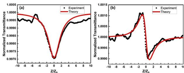
**Fig. 5** Measured normalized transmittance (black dotted curve) as a function of sample position for (a) open-aperture (OA) and (b) closed-aperture (CA) Z-scan experiment for complex **1**. The red solid curves are theoretical fits as per eqn (S6) and (S7)†.
