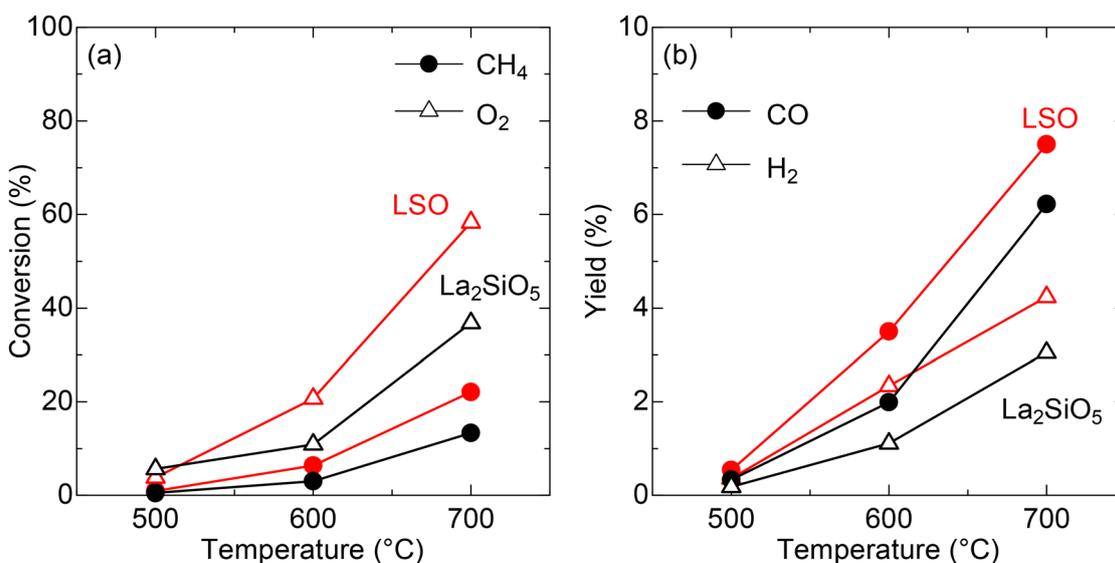
Fig. 5 (a) Catalytic conversions over LSO (red) and La<sub>2</sub>SiO<sub>5</sub> (black). Circles and triangles denote values for CH<sub>4</sub> and O<sub>2</sub>, respectively. (b) Catalytic yields over LSO (red) and La<sub>2</sub>SiO<sub>5</sub> (black). Circles and triangles denote values for CO and H<sub>2</sub>, respectively.
