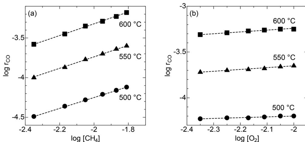
Fig. 6 Linear correlations between  $\log r_{\text{CO}}$  and (a)  $\log [\text{CH}_4]$  ( $\text{O}_2$  concentration: 12.5%) and (b)  $\log [\text{O}_2]$  ( $\text{CH}_4$  concentration: 25%) at 500, 550, and 600 °C. The total flow rate is set at  $10 \text{ mL min}^{-1}$ .
