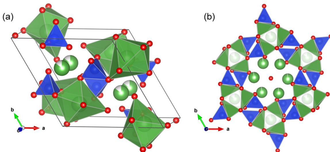
Fig. 2 (a) Schematic representation of the La<sub>9.33</sub>Si<sub>6</sub>O<sub>26</sub> apatite structure drawn with VESTA software.<sup>15</sup> (b) La and Si polyhedra enclose a one-dimensional tunnel containing mobile oxide ions (a red sphere in the middle). Color coding: green = La, blue = Si, red = O. Crystallographic data were extracted from ref. 16
