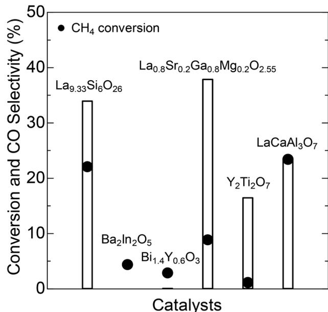
Fig. 1 CH<sub>4</sub> conversion and CO selectivity (at 700 °C) over various catalysts exhibiting oxide-ion-conductive capabilities.
