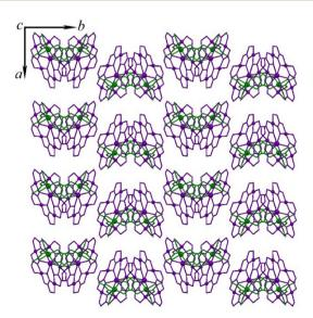
**Fig. 3** Fragment of the crystal structure of **1**, viewed along the *c*-direction. The 15-metallacrown-5 cations  $\{GdCu_5(GlyHA)_5\}^{3+}$  are presented in purple and  $[Cr(C_2O_4)_3]^{3-}$  anions are shown in green.
