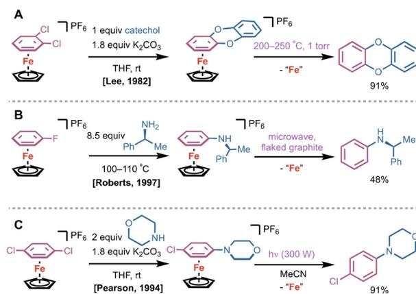
Fig. 2 (A) Lee and coworkers' synthesis of 9,10-dioxaanthracene using pyrolytic sublimation from the corresponding CpFe(II)( $\eta^6$ -arene). (B) Example of arene removal using flaked graphite in a microwave by Roberts. (C) Photolysis of a CpFe(II)( $\eta^6$ -arene) in MeCN solvent to yield desired *N*-aryl morpholine product.
