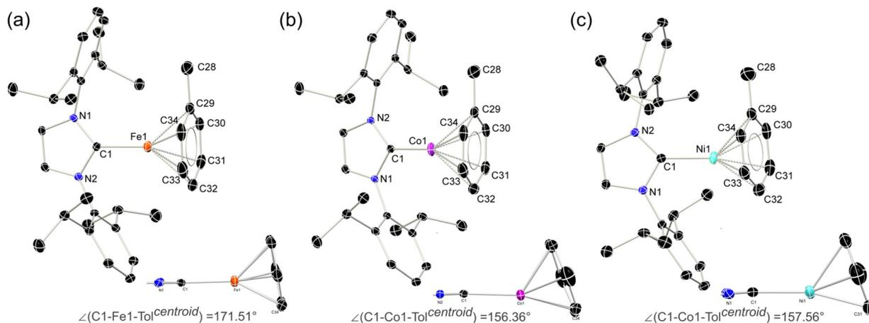
**Fig. 2** Molecular structure of the cationic part in (a) **1**, (b) **2**, and (c) **3**, with thermal ellipsoids at 30% probability, and hydrogen atoms removed for clarity. Inset: side-on view of the NHC–M–tol binding, demonstrating an increased tilt-angle in the C1–M–Tol<sup>centroid</sup> on moving from M = Fe to M = Ni.
