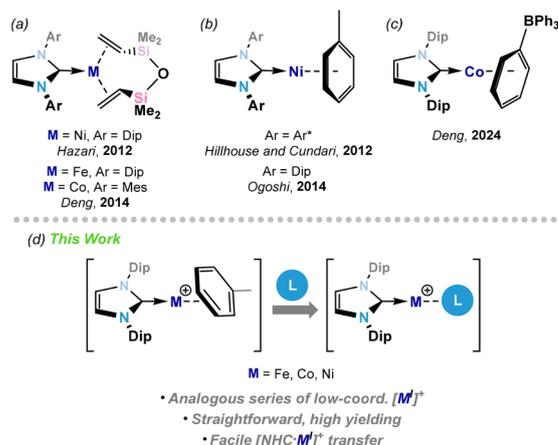
**Fig. 1** Key reported examples of (a) (dvtms)-complexes of NHC·M<sup>0</sup> moieties, (b) simple arene complexes of NHC·Ni<sup>0</sup> moieties, and (c) a cationic arene complex of Co<sup>I</sup>; (d) this work, demonstrating the facile access to arene adducts of cationic  $[\text{NHC}\cdot \text{M}^I]^+$  moieties, and their utility in  $[\text{NHC}\cdot \text{M}^I]^+$  group transfer.
