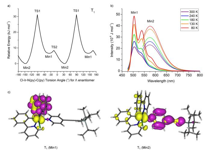
Fig. 6 (a) Relative triplet excited state  $(T_1)$  energies of 1 with respect to fixed Cl-Ir-N-C dihedral angles. (b) Simulated vibronic emission spectra from Min1 and Min2  $T_1$  optimised geometries. (c) Natural transition orbitals (NTO, purple = particle and yellow = hole) for Min1 and Min2  $T_1$  optimised geometries.
