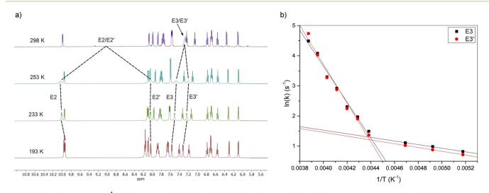
Fig. 2 (a) Variable temperature <sup>1</sup>H NMR spectra of 1 in THF-d<sub>8</sub>. (b) Arrhenius plot of the E3 and E3' proton signals recorded in THF-d<sub>8</sub>.
