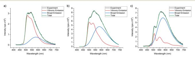
Fig. 5 Deconvolution curves from emission spectra of 1 in MeTHF at (a) 300 K, (b) 240 K and (c) 130 K.
