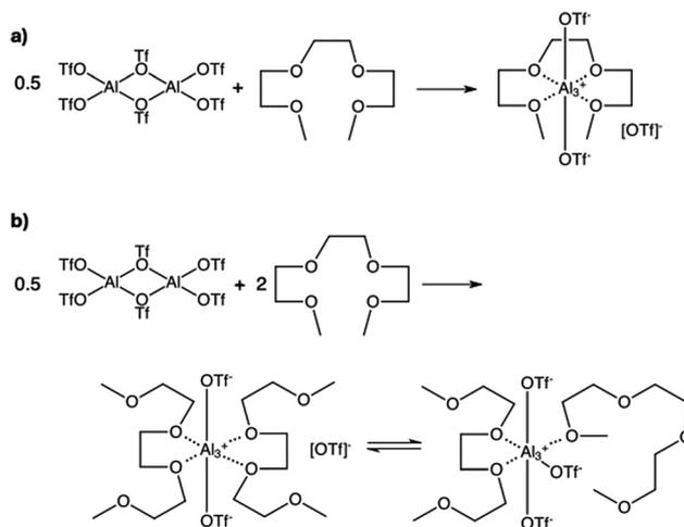
Fig. 2 Hypothetical speciation of Al-SILs synthesised at (a)  $\chi_{\text{M}(\text{OTf})_3} = 0.50$  (reaction did not proceed to completion) and (b)  $\chi_{\text{M}(\text{OTf})_3} = 0.33$  (reaction gave a homogeneous liquid).
