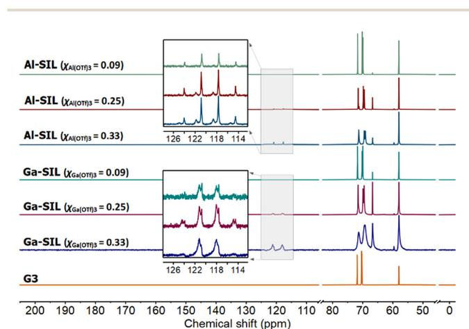
Fig. 5  $^{13}\text{C}$  NMR spectra of neat glyme, G3, and solvate ionic liquids based on  $\text{Al}(\text{OTf})_3$  or  $\text{Ga}(\text{OTf})_3$ , studied across three compositions:  $\chi_{M(OTf)_3} = 0.33, 0.25$  and  $0.09$ .
