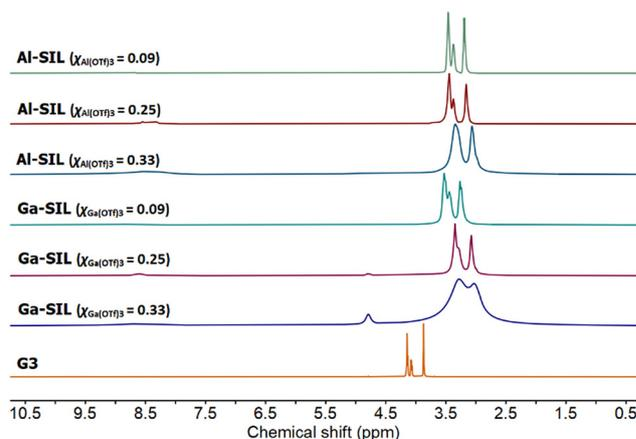
Fig. 4 <sup>1</sup>H NMR spectra of neat glyme, G3, and solvate ionic liquids based on Al(OTf)<sub>3</sub> or Ga(OTf)<sub>3</sub>, studied across three compositions:  $\chi_{M(OTf)_3} = 0.33, 0.25$  and 0.09.
