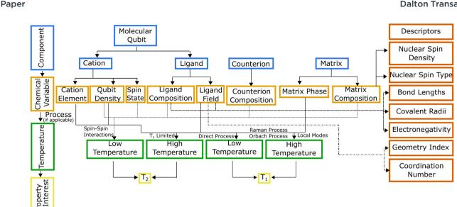
Fig. 1 Molecular qubit systems chart indicating how different components (blue) affect relaxation times (pale yellow) via changes to chemical variables (orange) in different temperature regimes (green). Annotations on lines connecting the chemical variables and temperature blocks indicate known spin relaxation processes that occur for the given chemical variable and temperature. Descriptors for chemical variables are shown in red.
