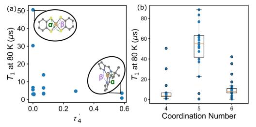
Fig. 4 (a)  $T_1$  at 80 K and  $\tau'_4$  for all 4-coordinate Cu molecules in the dataset. The molecular visualizations (inset) indicate the  $\alpha$  and  $\beta$  angles used to calculate  $\tau'_4$ . (b)  $T_1$  at 80 K and coordination number for all molecules in the data set.
