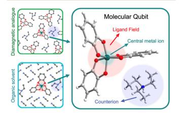
Fig. 2 Anatomy of a molecular qubit, prepared in either a diamagnetic host crystal (top left) or glassed in an organic solvent (bottom left). This example of  $[V(C_6H_4O_2)_7][Et_7NH]^{25}$  illustrates the central metal ion, organic ligands, and counterion that often constitute molecular gubits. V (dark green), carbon (gray), hydrogen (white), oxygen (red), nitrogen
