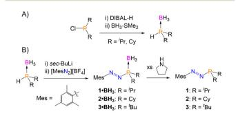
Scheme 1 (A) Synthesis of phosphine-borane precursors. (B) Synthesis of azophosphine-boranes and free azophosphines.
