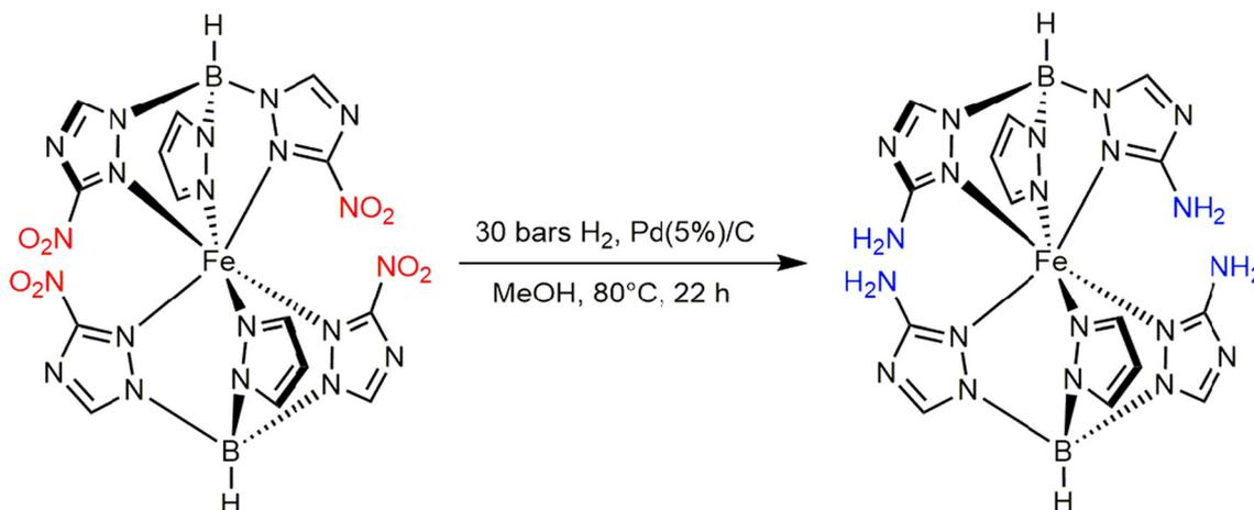
Fig. 2 Reduction of NO<sub>2</sub> groups in [Fe(L<sup>2</sup>)<sub>2</sub>].
