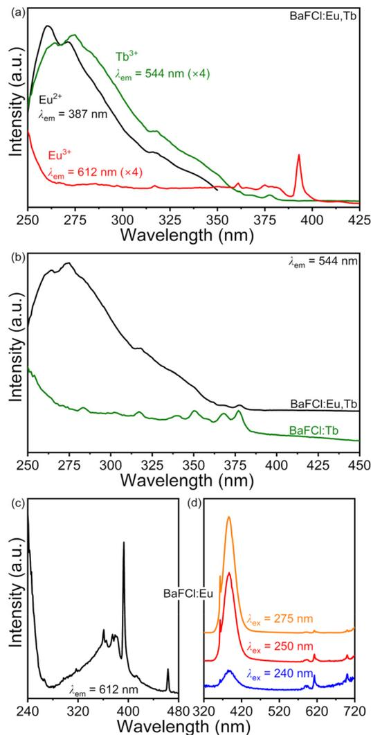
**Fig. 5** (a) Excitation spectra of BaFCl:Eu,Tb nanocrystals. (b) Excitation spectrum of BaFCl:Tb (6 mol%) nanocrystals. The spectrum of BaFCl:Eu, Tb is also shown to facilitate comparison. (c) and (d) show the excitation and emission spectra of BaFCl:Eu (6 mol%) nanocrystals. Spectra were collected at room temperature.
