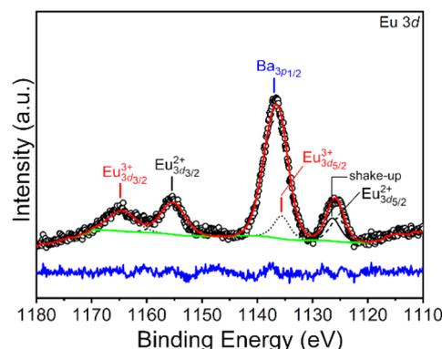
**Fig. 4** High-resolution Eu 3d XPS spectrum of BaFCl:Eu (4 mol%) nanocrystals. Experimental data (black circles), calculated spectrum (red line), background (green line), and difference curve (blue line, offset for clarity) are shown. Also shown are deconvoluted peaks corresponding to  $\text{Eu}^{2+}$  (short-dashed black line),  $\text{Eu}^{3+}$  (dotted black line), Ba 3p core (dashed black line), and shake-up features (solid black line).
