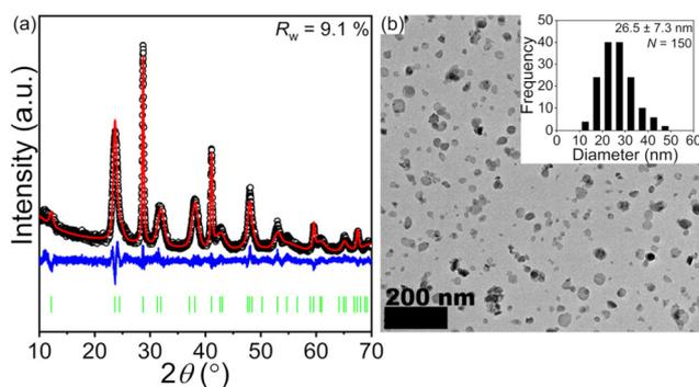
**Fig. 2** (a) Rietveld analysis of the PXRD pattern of BaFCl:Eu,Tb nanocrystals. Experimental data (black circles), calculated pattern (red line), difference curve (blue line, offset for clarity), and tick marks corresponding to the calculated diffraction maxima are shown (green vertical bars). (b) Electron microscopy image and nanocrystal size distribution histogram (inset).
