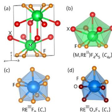
**Fig. 1** (a) Unit cell of matlockite MFX. (b) Coordination polyhedra of divalent metals in the matlockite structure. (c and d) Possible coordination polyhedra of trivalent rare-earth metals.<sup>22</sup> Point group symmetries are indicated for each polyhedron.
