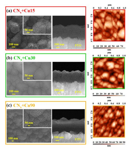
Fig. 6 Representative plane-view (left panel) and cross-sectional (central panel) FE-SEM images for the  $CN_x + Cu15$  (a),  $CN_x + Cu30$  (b),  $CN_x + Cu90$  samples (c). Right panel: AFM micrographs for the same specimens.
