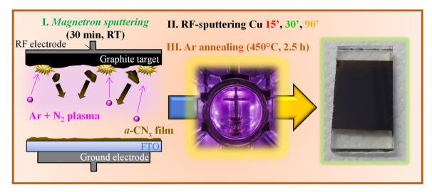
Fig. 1 Sketch of the preparation of a-CN<sub>x</sub>-based electrodes functionalized with Cu<sub>x</sub>O nanoparticles: (I) magnetron sputtering from a graphite target in an Ar + N<sub>2</sub> plasma; (II) RF-sputtering of Cu<sub>x</sub>O nanoclusters from a Cu target in an Ar plasma, and (III) thermal treatment under an Ar
