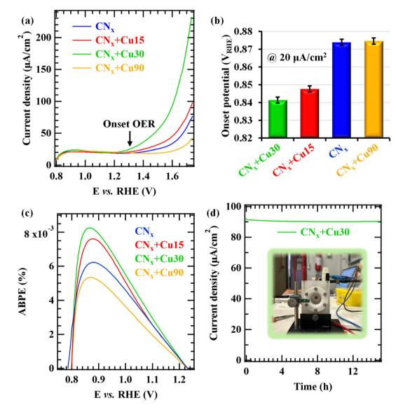
Fig. 10 (a) LSV curves recorded under illumination; (b) onset potentials and (c) ABPE (%) curves for the bare  $CN_x$  and  $Cu_xO$ -functionalized samples; and (d) chronoamperometry test for  $CN_x + Cu30$  collected under irradiation at 1.60 V vs. RHE for 15 h (inset: photograph of the used apparatus).
