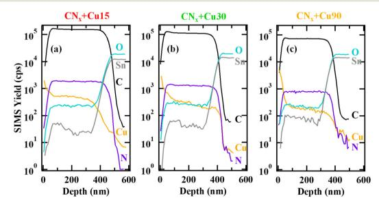
Fig. 4 SIMS depth profiles for CN<sub>x</sub> + Cu15 (a), CN<sub>x</sub> + Cu30 (b), CN<sub>x</sub> + Cu90 (c). The deposit thickness ranged from 460 nm, for CN<sub>x</sub> + Cu15, to 370 nm, for  $CN_x + Cu90$  (uncertainty =  $\pm 30$  nm).
