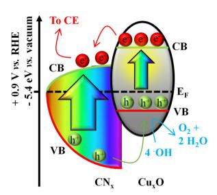
**Fig. 11** Approximate band diagram for the  $CN_x/Cu_xO$  heterojunction. The positions of VB (valence band) and CB (conduction band) edges for a- $CN_x$  are represented by red and green curves, respectively. The VB-CB edge separation for  $CN_x$  is proposed considering the  $E_G$  values reported in Fig. 2. The Fermi level ( $E_F$ ) position on the vacuum scale was deduced from the work function values reported in Fig. S7.†
