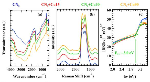
Fig. 2 (a) FT-IR spectra, (b) Raman spectra, and (c) Tauc plots (obtained from the optical spectra in Fig. S2†) of the target specimens.
