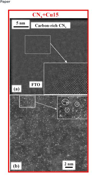
Fig. 7 (a) High-resolution HAADF-STEM image of the FTO/CN<sub>x</sub> interface for the  $CN_x$  + Cu15 sample. The area framed by the white box is magnified in the inset. (b) Cross-sectional high resolution HAADF-STEM image of the Cu<sub>x</sub>O-rich region. The white circles in the magnified inset image mark ultra-dispersed, "quasi-atomic" Cu<sub>x</sub>O.
