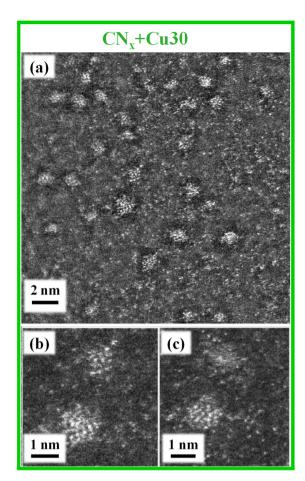
Fig. 8 (a) Cross-sectional high-resolution HAADF-STEM image of the CN<sub>x</sub> + Cu30 sample. (b and c) Representative high-resolution HAADF-STEM images.
