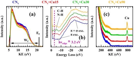
Fig. 5 (a) UPS work function determination for the indicated specimens ( $W_f$  = work function); (b) REELS spectra showing the presence of the  $\pi$  and  $\pi + \sigma$  plasmonic excitation typical of such composite materials. The incorporation of H and N atoms is evidenced by the small peak centred at  $\approx$ 1.98 eV, while the optical band gap is estimated at  $\approx$ 3.2 eV. (c) ISS spectra highlighting the different Cu<sub>x</sub>O surface contents for the composite samples.
