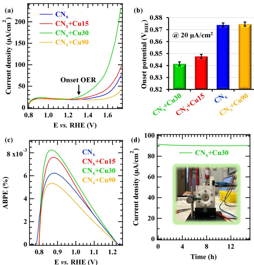
Fig. 10 (a) LSV curves recorded under illumination; (b) onset potentials and (c) ABPE (%) curves for the bare  $\text{CN}_x$  and  $\text{Cu}_x\text{O}$ -functionalized samples; and (d) chronoamperometry test for  $\text{CN}_x + \text{Cu}30$  collected under irradiation at 1.60 V vs. RHE for 15 h (inset: photograph of the used apparatus).
