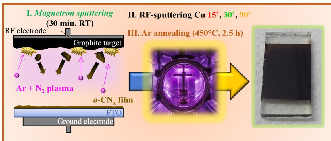
**Fig. 1** Sketch of the preparation of a-CN<sub>x</sub>-based electrodes functionalized with Cu<sub>x</sub>O nanoparticles: (I) magnetron sputtering from a graphite target in an Ar + N<sub>2</sub> plasma; (II) RF-sputtering of Cu<sub>x</sub>O nanoclusters from a Cu target in an Ar plasma, and (III) thermal treatment under an Ar atmosphere.
