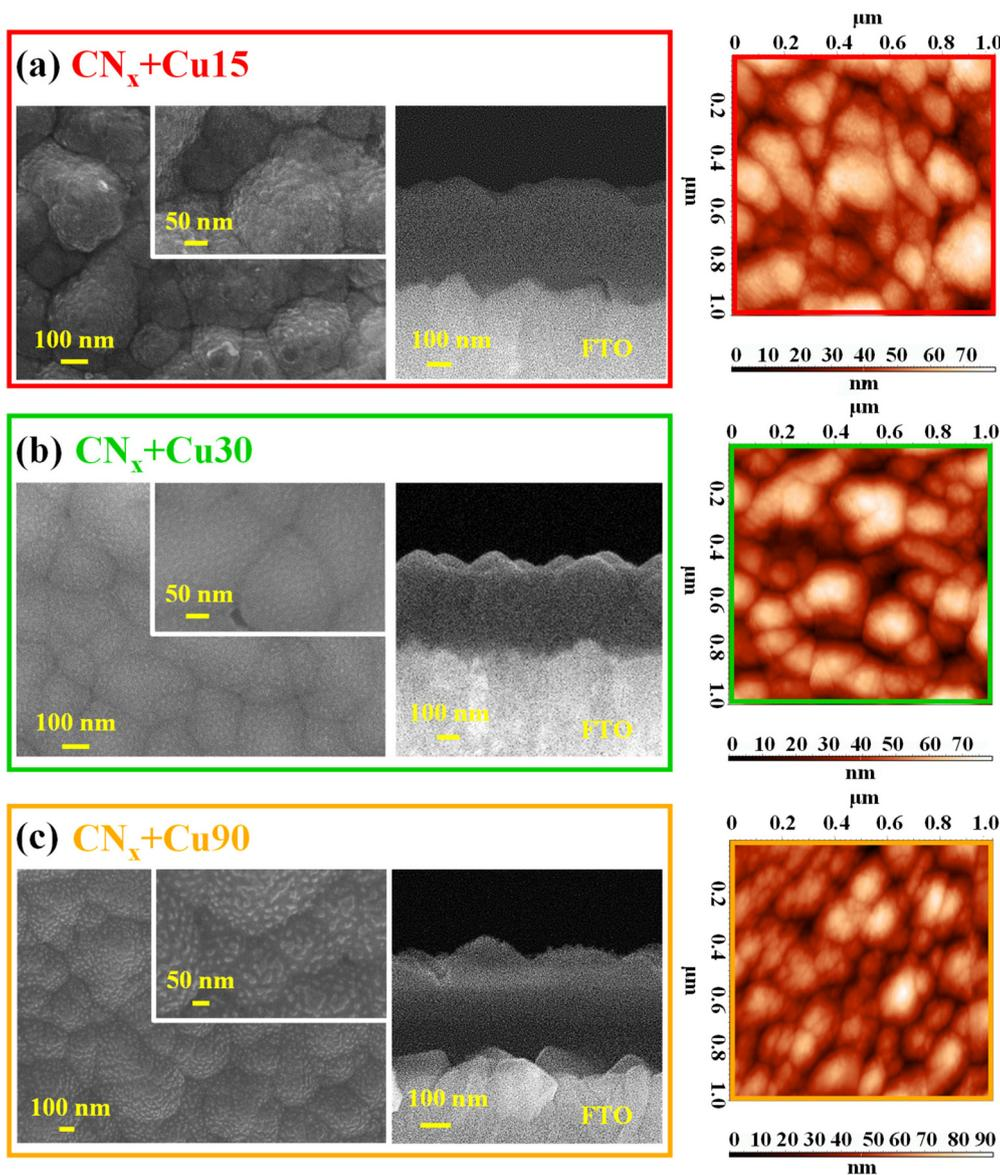
Fig. 6 Representative plane-view (left panel) and cross-sectional (central panel) FE-SEM images for the  $\text{CN}_x + \text{Cu}15$  (a),  $\text{CN}_x + \text{Cu}30$  (b),  $\text{CN}_x + \text{Cu}90$  samples (c). Right panel: AFM micrographs for the same specimens.
