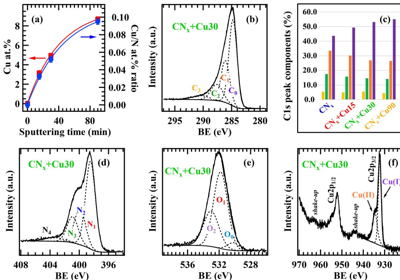
Fig. 3 (a) Cu at.% and Cu/N atomic ratio vs. sputtering time (Cu at.% was calculated excluding C and O). (b) Deconvoluted C 1s peak for the  $\text{CN}_x + \text{Cu30}$  specimen. (c) Trend of the various C 1s peak components for the bare  $\text{CN}_x$  and  $\text{Cu}_x\text{O}$ -functionalized samples, color codes are the same used for the C 1s bands in (b). (d) N 1s, (e) O 1s, and (f) Cu 2p photopeaks for the  $\text{CN}_x + \text{Cu30}$  sample.
