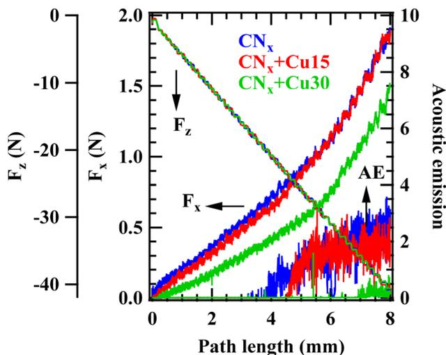
Fig. 9 Scratch test outputs from selected  $\text{CN}_x$  and  $\text{CN}_x + \text{Cu}$  samples.
