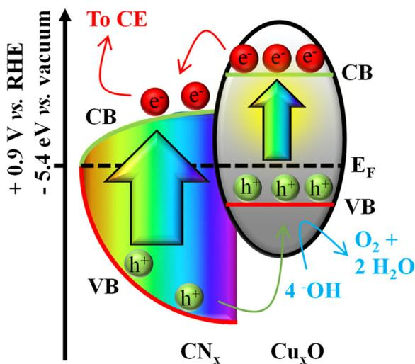
**Fig. 11** Approximate band diagram for the  $\text{CN}_x/\text{Cu}_2\text{O}$  heterojunction. The positions of VB (valence band) and CB (conduction band) edges for a- $\text{CN}_x$  are represented by red and green curves, respectively. The VB–CB edge separation for  $\text{CN}_x$  is proposed considering the  $E_G$  values reported in Fig. 2. The Fermi level ( $E_F$ ) position on the vacuum scale was deduced from the work function values reported in Fig. S7.†
