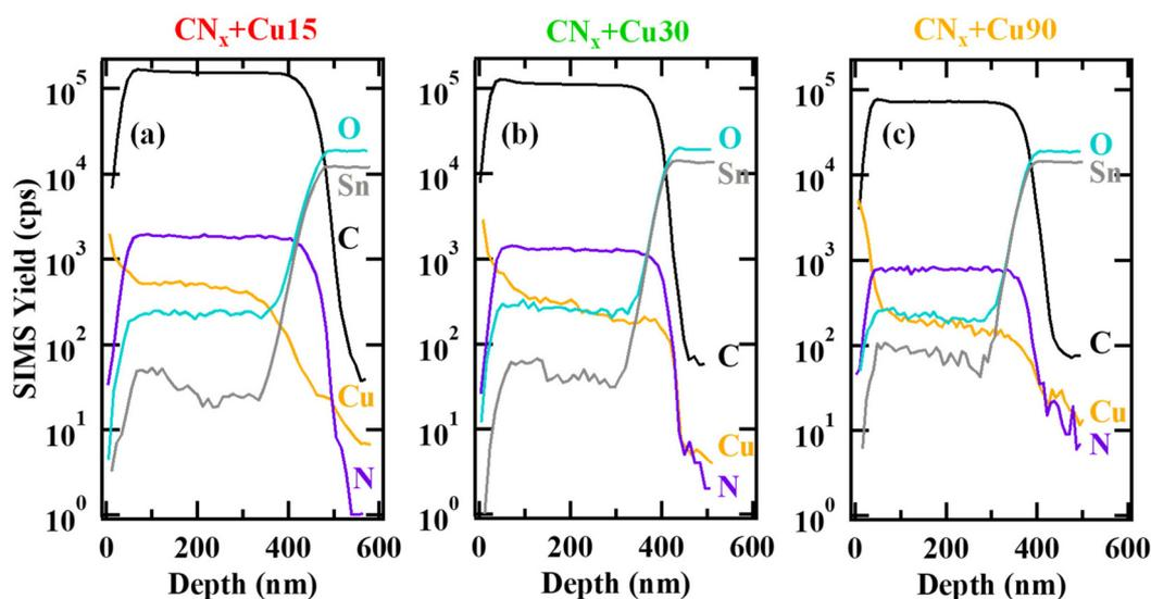
Fig. 4 SIMS depth profiles for CN<sub>x</sub> + Cu15 (a), CN<sub>x</sub> + Cu30 (b), CN<sub>x</sub> + Cu90 (c). The deposit thickness ranged from 460 nm, for CN<sub>x</sub> + Cu15, to 370 nm, for CN<sub>x</sub> + Cu90 (uncertainty = ±30 nm).
