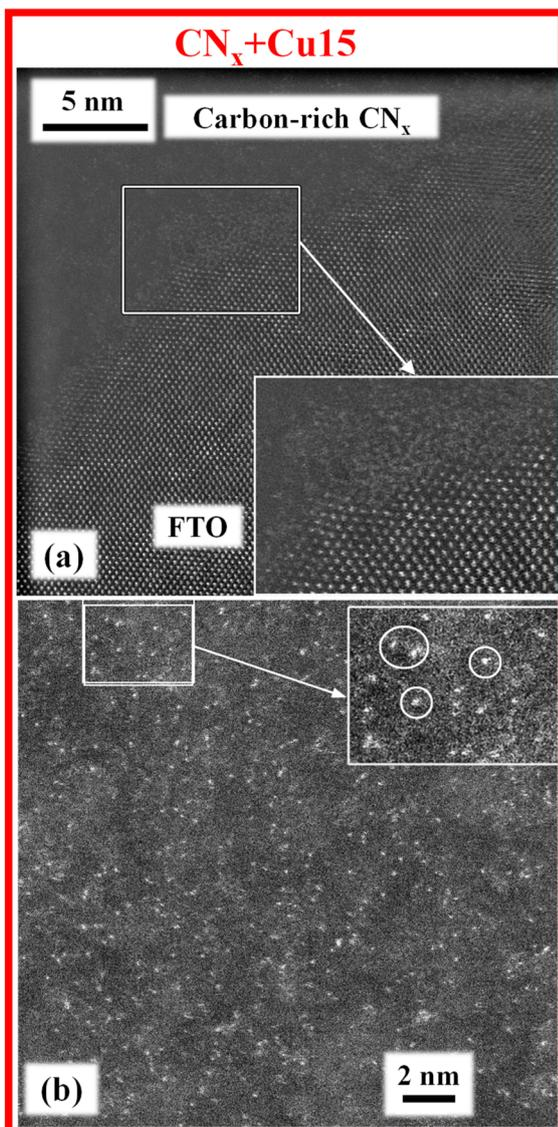
**Fig. 7** (a) High-resolution HAADF-STEM image of the FTO/ $\text{CN}_x$  interface for the  $\text{CN}_x + \text{Cu15}$  sample. The area framed by the white box is magnified in the inset. (b) Cross-sectional high resolution HAADF-STEM image of the  $\text{Cu}_2\text{O}$ -rich region. The white circles in the magnified inset image mark ultra-dispersed, "quasi-atomic"  $\text{Cu}_2\text{O}$ .
