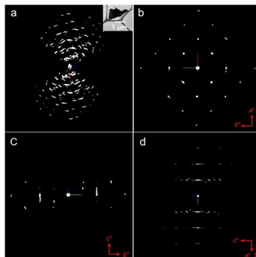
Fig. 3 The reconstructed 3D reciprocal lattice of BiOBr-1 (an inset is an image of the crystal from which the cRED data was collected) and 2D slice cuts show the  $hk0$  (b),  $0kl$  (c), and the (d) planes.
