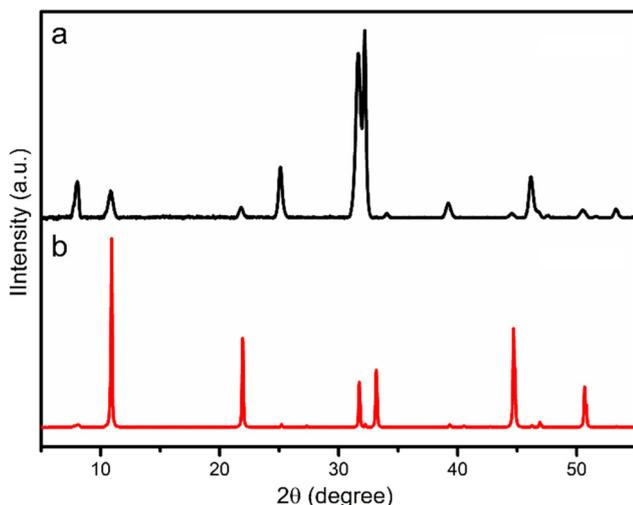
Fig. 2 XRD patterns for (a) BiOBr-1 and (b) BiOBr-2.
