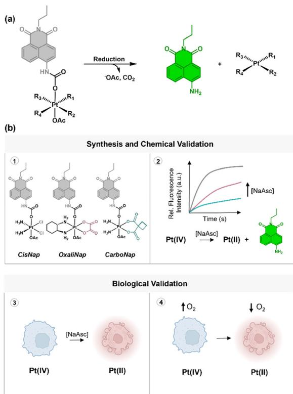
**Fig. 1** (a) General schematic showing the reduction of a fluorogenic Pt(IV) complex to Pt(II) and release of the Nap-NH<sub>2</sub> (green) fluorophore; (b) the proposed stepwise workflow using fluorogenic Pt(IV) systems to aid the general development of a HAPT: (1) chemical synthesis; (2) chemical validation using NaAsc; (3) chemical reduction in cells using NaAsc; and (4) anaerobic reduction in cells using decreased oxygen concentrations.
