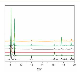
Fig. 1 PXRD patterns of the  $Gd-F_4BDC$  MOF obtained through the synthetic procedure reported: synthesis no. 1 (olive green), synthesis no. 2 (red line), synthesis no. 3 (grey line), synthesis no. 4 (orange), and synthesis no. 5 (light green). The calculated PXRD pattern is also reported (black line).
