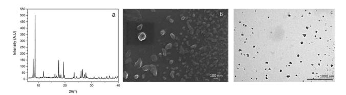
Fig. 3 PXRD patterns of the Gd-F<sub>4</sub>BDC MOF NPs are shown in (a) (acetic acid was used as a modulator) whereas (b) and (c) show selected SEM and TEM images. Other images are reported in Fig. S4 and S5 (ESI†).
