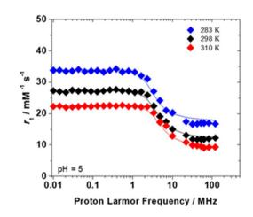
Fig. 4 1H  $T_1$  NMRD profiles of the Gd-F<sub>4</sub>BDC MOF ([Gd<sup>3+</sup>] = 4.77 mM) at 283, 298, and 310 K.
