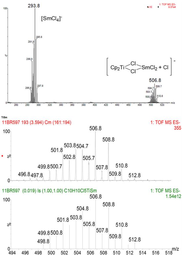
Fig. 1 ESI-MS spectrum (negative mode) for the reduction of  $\text{Cp}_2\text{TiCl}_2$  with Sm in THF (above); observed (middle) vs. calculated (bottom) isotope distribution of the bimetallic complex.
