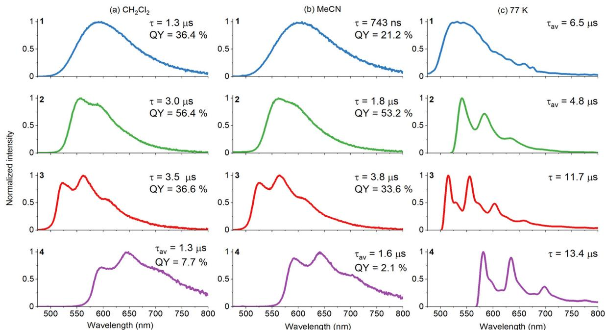
**Fig. 5** Emission spectra of compounds 1–4 in CH<sub>2</sub>Cl<sub>2</sub>, MeCN, and an EtOH : MeOH (4 : 1 v/v) rigid matrix at 77 K, along with their respective photoluminescence lifetimes and quantum yields. For samples with decay profiles fitted to biexponential functions, average lifetime values  $\tau_{av}$  were given (see also Fig. S21–S24†).
