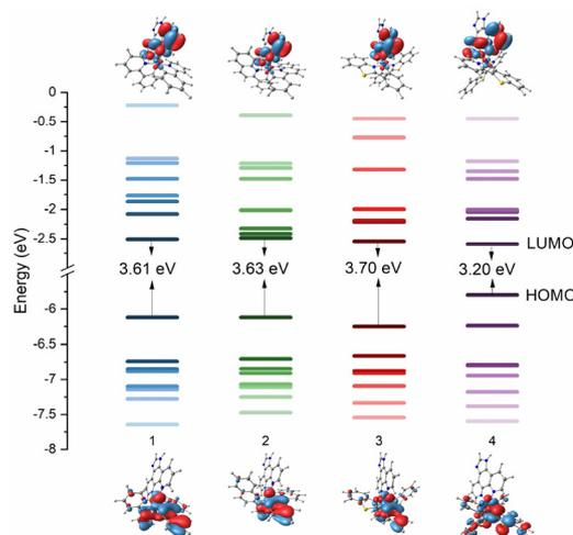
**Fig. 2** Partial molecular orbital energy level diagram with the plots of electron density distributions in the HOMO (below) and the LUMO (above) of 1–4 (see also Fig. S7–S10<sup>†</sup>).
