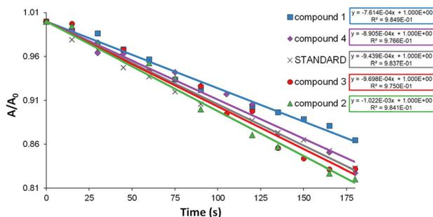
**Fig. 10** Plots of  $A/A_0$  against the irradiation time for the photooxidation reaction of DPBF using Ir(III) complexes (1–4) and  $[\text{Ru}(\text{bipy})_3](\text{PF}_6)_2$  as sensitizers.  $A_0$  and  $A$  stand for absorbance at  $t = 0$  s and after the given irradiation time, respectively.
