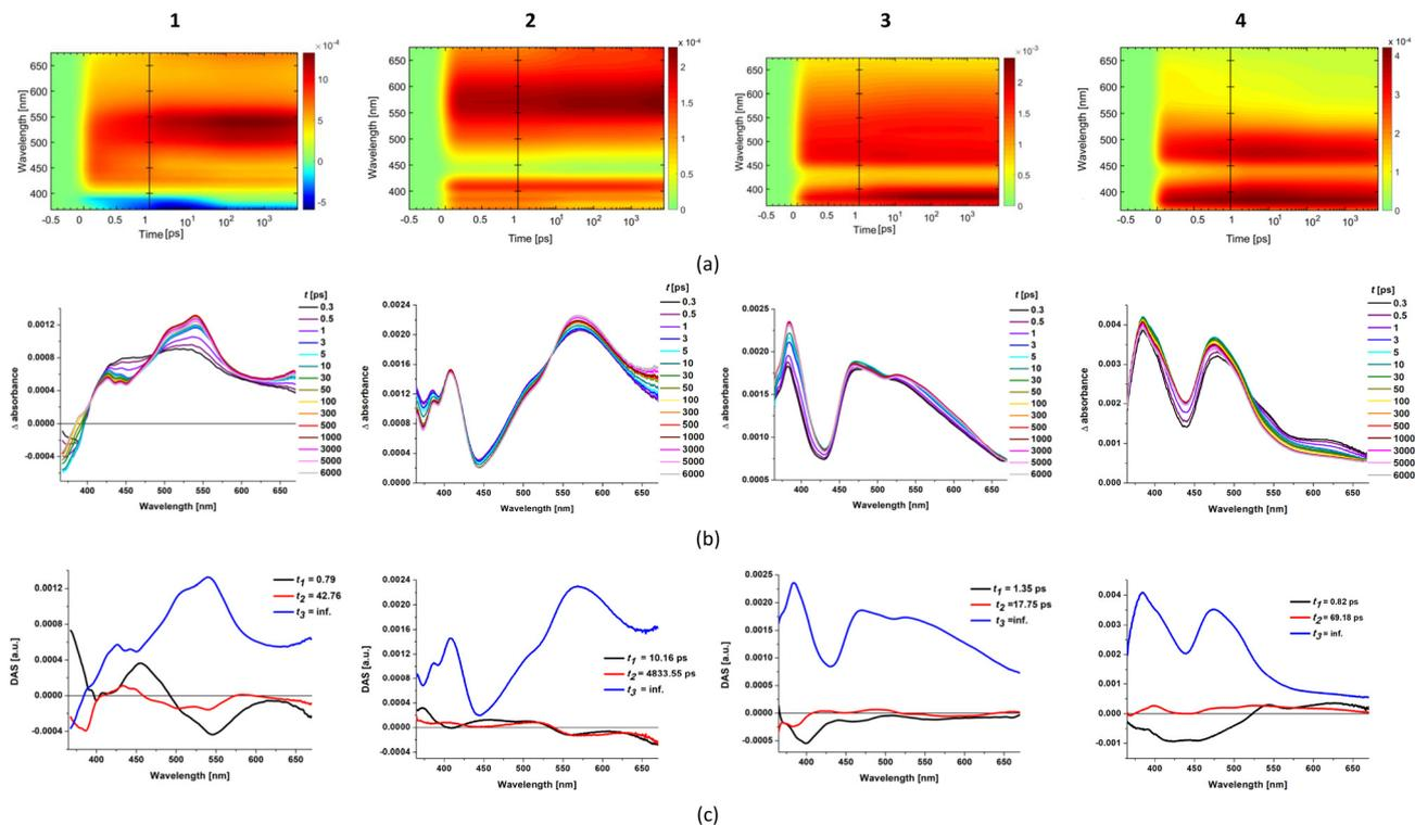
**Fig. 8** The results of fs-TA measurements and global fitting analyses of **1–4**: (a) 2D time–wavelength plots; (b) fs-TA spectra at selected time delays (ps); and (c) decay-associated spectra DAS, with appropriate time constants  $t_i$  (see also Fig. S29–S32†).
