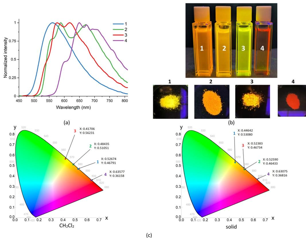
**Fig. 6** Solid-state emission spectra of complexes 1–4 (a). Photographs of CH<sub>2</sub>Cl<sub>2</sub> solutions and the solid samples of compounds 1–4 under UV light (b), along with their CIE 1931 chromaticity plots (c).
