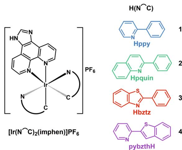
**Scheme 1** Discussed iridium(III) complexes 1–4. H(NΩC) stands for different cyclometalating ligands: Hppy – 2-phenylpyridine, Hpquin – 2-phenylquinoline, Hpbztz – 2-phenylbenzothiazole, and pybztzH – 2-(2-pyridyl)benzothiophene.
