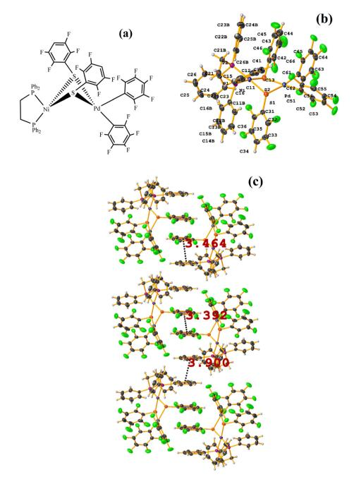
Fig. 23 (a) Schematization of the molecular structure WUNRAY. (b) Molecular structure of WUNRAY. (c) Supramolecular array of WUNRAY.
