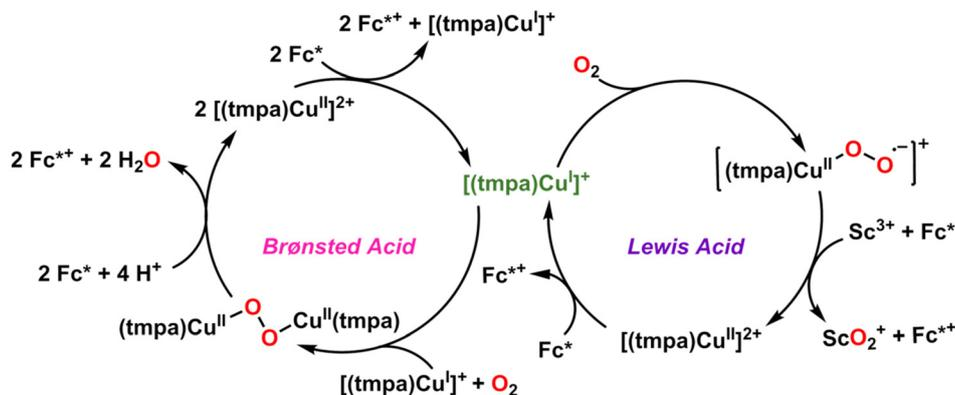
**Fig. 5** Proposed catalytic cycles for the reduction of dioxygen by [Cu<sup>II</sup>(tmpa)(CH<sub>3</sub>CN)](HClO<sub>4</sub>)<sub>2</sub>, where (tmpa = tris(2-pyridylmethyl)amine), in the presence of Brønsted Acids (left) and Lewis Acids (right). The mechanistic differences between the two cycles result in a quantitative shift in selectivity from water (Brønsted) to hydrogen peroxide (Lewis). Adapted from ref. 47 and 48.
