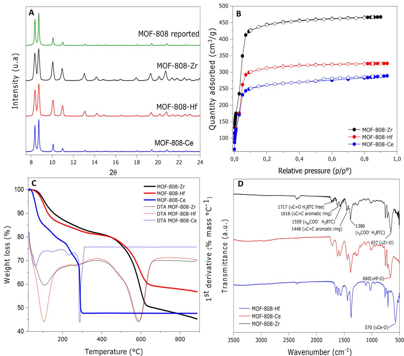
**Fig. 1** Characterization obtained for MOF-808-Zr, MOF-808-Hf and MOF-808-Ce; (A) PXRD patterns; (B) TGA analysis; (C) nitrogen adsorption-desorption isotherm and (D) ATR-FTIR spectra.
