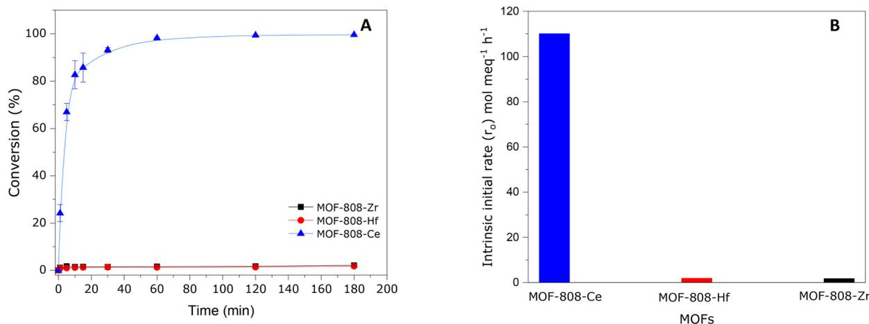
**Fig. 5** Conversion versus time in the acetalization of benzaldehyde with methanol catalyzed by MOF-808-Zr, MOF-808-Hf and MOF-808-Ce (A), intrinsic initial rate for MOF-808-Zr, MOF-808-Hf and MOF-808-Ce normalizing by ASD (B).
