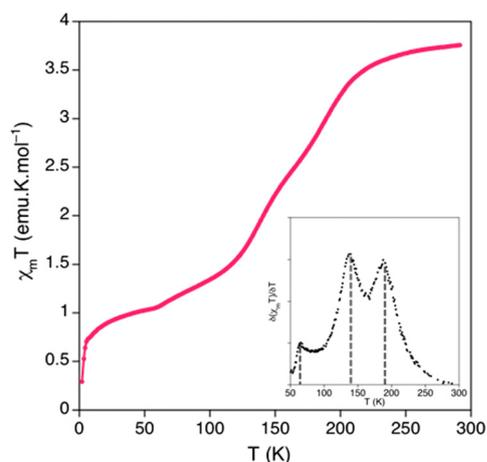
**Fig. 8** Magnetic data for  $[\text{Fe}(\mu\text{-btix})_{0.6}(\mu\text{-btzx})_{2.4}][\text{ClO}_4]_2$  (Scheme 6), and (inset) the first derivative of the data highlighting the three components in its SCO. This figure has been adapted from ref. 146 with permission from the American Chemical Society, copyright 2014.
