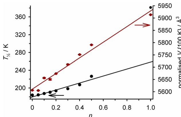
**Fig. 10** Composition dependence of  $T_{\frac{1}{2}}$  (black) and the normalised unit cell volume at 100 K (red) in  $[\text{Fe}(\text{Me}_2\text{1,3-bpp})_{2n}(\text{Me1,3-bpp})_{2-2n}][\text{ClO}_4]_2$  (Scheme 8).<sup>123</sup> Both plots are connected by regression lines for clarity. The data are replotted from ref. 129 and 148.
