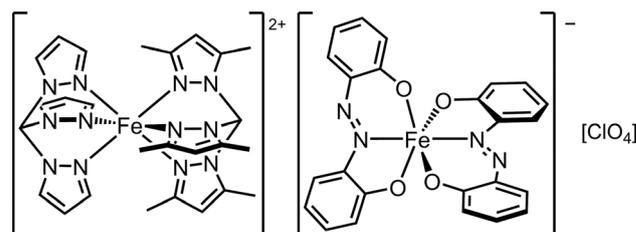
**Scheme 5** The  $[\text{Fe}^{\text{II}}(\text{tpm})(\text{tpm}')][\text{Fe}^{\text{III}}(\text{azp})_2]\text{ClO}_4$  SCO double salt.<sup>130</sup>
