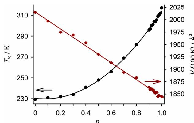
**Fig. 9** Composition dependence of  $T_{\frac{1}{2}}$  (black) and the crystallographic unit cell volume at 100 K (red) in  $[\text{Fe}(\text{H}_{0.5}\text{L}^{\text{F}})_{2n}(\text{H}_{0.5}\text{L}^{\text{Cl}})_{2-2n}] \cdot \text{H}_2\text{O}$  (Scheme 7). Both plots are connected by regression lines for clarity. The data are replotted from ref. 128.
