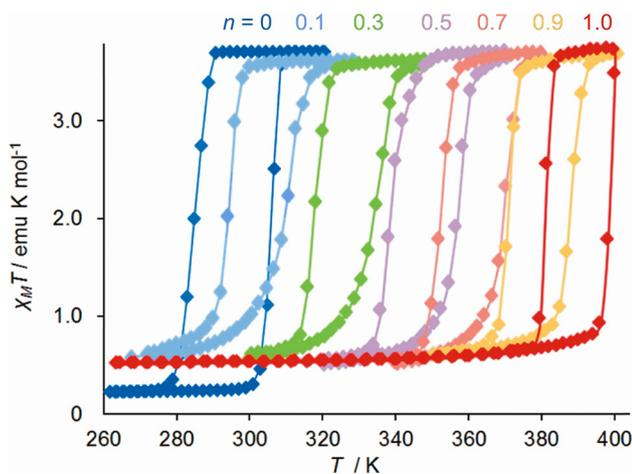
Fig. 11 Magnetic data from six compositions of  $[\text{Fe}(\mu\text{-pyz})\{\text{PtI}_2(\text{CN})_4\}_n\{\text{Pt}(\text{CN})_4\}_{1-n}]$ . This figure has been adapted from ref. 158 with permission from the American Chemical Society, copyright 2011.
