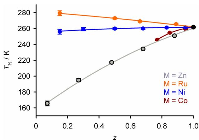
**Fig. 3** Variation of  $T_{1/2}$  with composition in  $[\text{Fe}_z\text{M}_{1-z}(1\text{-bpp})_2][\text{BF}_4]_2$  (Scheme 1) with different dopant ions. The  $\text{Fe}_z\text{Zn}_{1-z}$  data correspond to those in Fig. 2. Analogous data for other doped SCO compounds are in Fig. S1 and S2.† This figure has been adapted from ref. 63 with permission from the Royal Society of Chemistry, copyright 2023.
