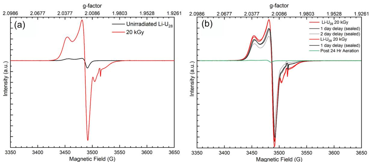
**Fig. 5** (a) EPR spectra of solid Li-U<sub>28</sub> unirradiated (black) and 20 kGy  $\gamma$ -irradiated (red). (b) EPR spectra tracking radical decay over two days. Li-U<sub>28</sub> 20 kGy (red), Li-U<sub>28</sub> one day after 20 kGy  $\gamma$ -irradiation sealed (black), Li-U<sub>28</sub> two days after 20 kGy  $\gamma$ -irradiation sealed (gray), Li-U<sub>28</sub> two days after  $\gamma$ -irradiation and 24 hours after exposure to air (green).
