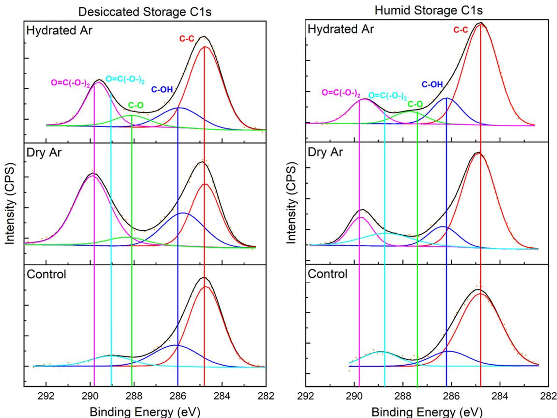
**Fig. 4** XPS spectra of the C 1s binding envelopes. Li-U<sub>28</sub> stored in desiccated environment (left) Li-U<sub>28</sub> stored in 75% RH environment (right). From top to bottom: Li-U<sub>28</sub> He<sup>2+</sup> irradiated to 42 MGy under hydrated Ar flow, Li-U<sub>28</sub> irradiated to 42 MGy under dry Ar flow, unirradiated Li-U<sub>28</sub> controls kept in respective storage environments.
