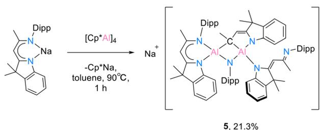
**Scheme 5** Reaction of solvent-free  $[\text{DNINa}]$  with  $[(\text{Cp}^*\text{Al})_4]$  (**B**).
