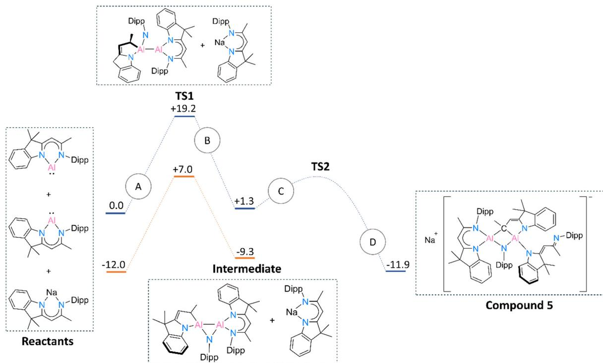
**Fig. 6** Reaction path for obtaining compound **5** and corresponding free energies (kcal mol<sup>-1</sup>) of the reactants in the gas phase. Blue lines represent the gas phase route, whereas the orange lines depict the reaction in the toluene solvated medium. Transition state 2 could not be reliably defined. The meaning of A, B, C and D paths is described in the ESI† file (see the Computational details section).
