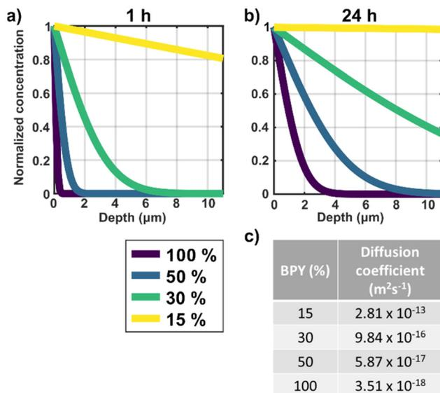
**Fig. 7** Depth-dependent  $Ni^{2+}$  concentration in four mixed-linker UiO-67-BPY MOFs (15–100% BPY) after (a) 1 hour, and (b) 24 hours metalation. The graphs were obtained by plotting diffusion functions using the different diffusion coefficients presented in (c) table of Fickian  $Ni^{2+}$  diffusion coefficients extracted from fitting the RBS spectra of the different mixed-linker crystals metalated for one hour (from Fig. 6).
