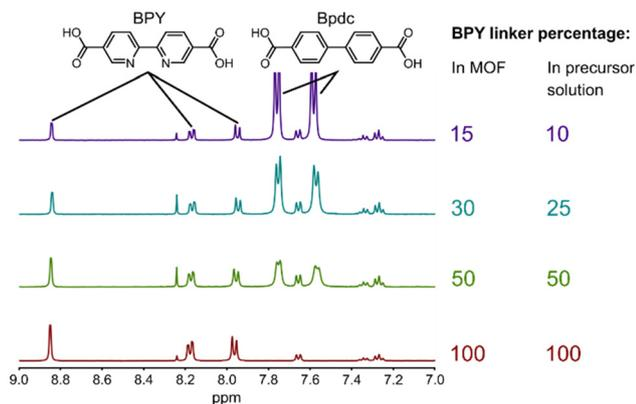
**Fig. 3** NMR spectra of digested UiO-67 crystals containing different percentages of BPY linker. The table shows the BPY percentage in the precursor solution compared to the measured BPY percentage in the digested MOF crystals. BPY percentage values were rounded to multiples of 5.
