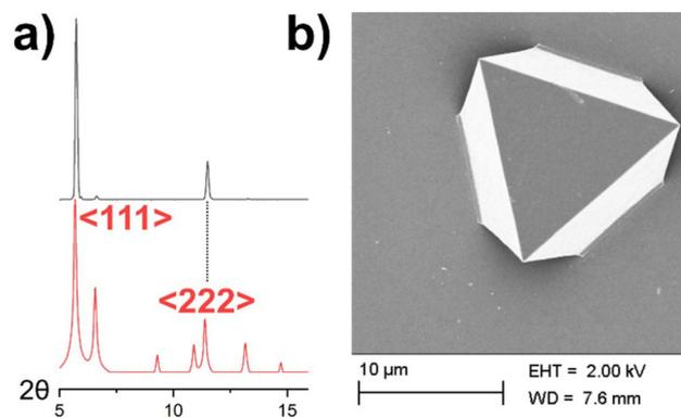
Fig. 2 (a) In black, a measured XRD pattern of synthesized UiO-67-BPY<sub>100%</sub> crystals displaying only the <111> and <222> reflections; in red a simulated XRD spectrum of non-oriented UiO-67 crystals. (b) SEM picture of a synthesized UiO-67-BPY<sub>100%</sub> crystal on a Si substrate.
