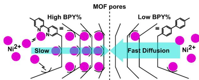
Fig. 1 Schematic representation of Ni<sup>2+</sup> cations entering a MOF with high (left) and low (right) BPY content.
