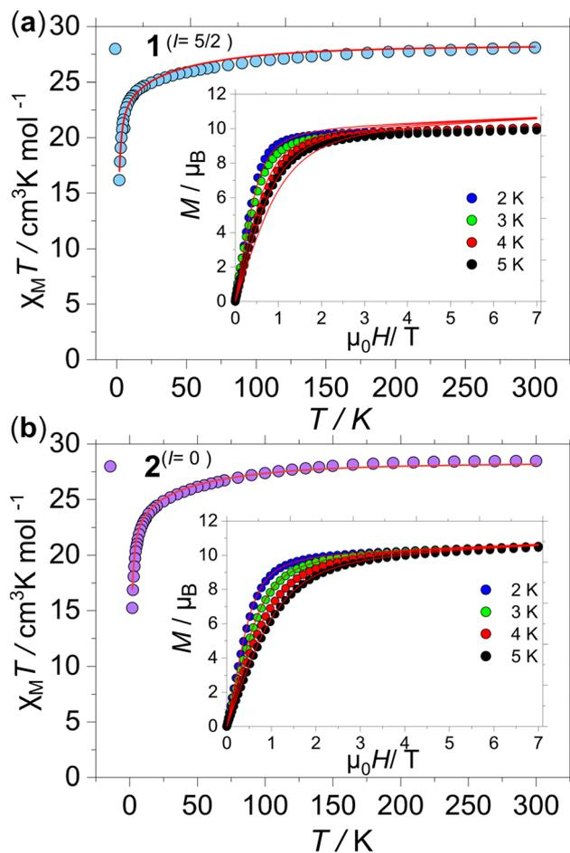
Fig. 2 The  $\chi_{\text{M}}T$  vs.  $T$  plots for compounds (a)  $\mathbf{1}^{(f=5/2)}$  and (b)  $\mathbf{2}^{(f=0)}$ . Inset:  $M(H)$  data at different temperatures. Solid lines are the fits using the CF parameters obtained from CASSCF calculations as described in the main text.
