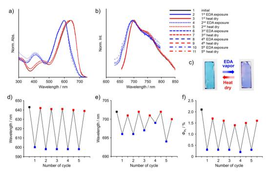
Fig. 7 Reversible controls of (a and d) UV-vis absorption, (b and e) PL properties, (c) photographs under room right, and (f) absolute PL quantum yields of P-TAz in film upon exposure to EDA vapor and dry processes (80 °C for 3 min on the hot plate). The detailed method and spectroscopic data are shown in Fig. S9 and Table S5,† respectively.
