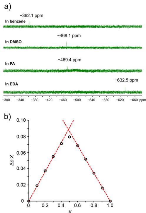
**Fig. 1** (a)  $^{119}\text{Sn}$  NMR spectra of **TAz** in benzene, DMSO, PA and EDA. (b) The  $^1\text{H}$  NMR Job plot for the binding of **TAz** with EDA (total concentration = 10 mM) in benzene- $d_6$ .
