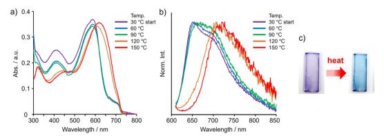
Fig. 8 (a) Changes in UV-vis absorption and (b) PL spectra by heating and (c) photographs of theremochromic behaviors of the film containing P-TAz and phen under room light.
