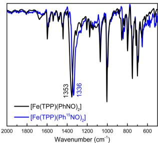
Fig. 1 Top panel: Overlay of the IR spectra of [Fe(TPP)(THF)(PhNO)] (black), and of the  $^{15}$ N-labeled complex, [Fe(TPP)(THF)(Ph $^{15}$ NO)] (green), measured in KBr pellets (expanded view of the N–O stretching frequency region). Bottom panel: Overlay of the IR spectra of [Fe(TPP)(PhNO)<sub>2</sub>] (black) and the  $^{15}$ N-labeled complex, [Fe(TPP)(Ph $^{15}$ NO)<sub>2</sub>] (blue), measured in KBr pellets. See text for further discussion.
