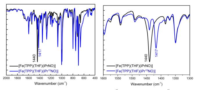
Fig. 3 Left panel: Overlay of the IR spectra of [Fe(TPP)(THF)(iPrNO)] (black) and of the <sup>15</sup>N-labeled complex, [Fe(TPP)(THF)(iPr<sup>15</sup>NO)] (blue). The data were obtained in KBr pellets. Right panel: Expanded region of the N-O stretching frequency. The natural abundance isotopes (n.a.i.) complex [Fe (TPP)(THF)(iPrNO)] has one isotope sensitive feature at 1440 cm<sup>-1</sup> that shifts to 1417 cm<sup>-1</sup> upon <sup>15</sup>N-labeling.
