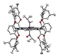
Fig. 9 Crystal structure of [Fe(3.5-Me-BAFP)(iPrNH<sub>2</sub>)(iPrNO)]. Hydrogen atoms, except for the amine group of iPrNH2, are omitted for clarity. Thermal ellipsoids are shown at 50% probability.
