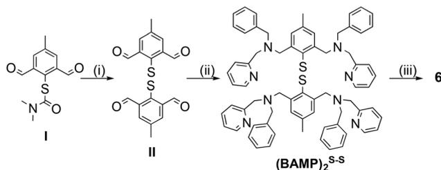
Fig. 2 Preparation of the  $(\text{BAMP})_2^{\text{S-S}}$  ligand from (**I**)<sup>30</sup> and metalation into **6**.
