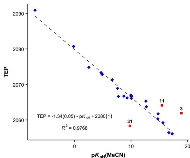
Fig. 4 Correlation between  $pK_{aH}(\text{MeCN})$  values and TEP values. Blue diamonds: datapoints included in the correlation denoted by a dashed line; red squares: points omitted from the correlation (outliers according to the Grubbs test).
