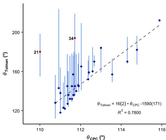
**Fig. 6** Correlation between CPC and Tolman angles. Blue diamonds: datapoints included in the correlation denoted by a dashed line; red squares: points omitted from the correlation (outliers according to the Grubbs test). Vertical bars show ranges of various cone angles reported in the literature, including solid cone angle.<sup>9,30,37</sup>
