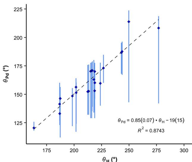
**Fig. 8** Correlation between the average exact cone angle of palladium complexes and the exact cone angle of the cation with hydrogen as the apex. Vertical bars show the range of various cone angles reported in the literature, including solid cone angle.<sup>9,30,37</sup>
