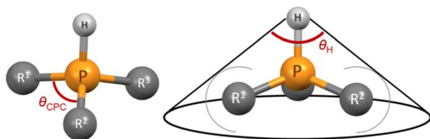
**Fig. 5** Single CPC angle (left); the average CPC angle used in this work is calculated using all three single CPC angles.  $\theta_{\text{H}}$  angle (right) of a phosphine.
