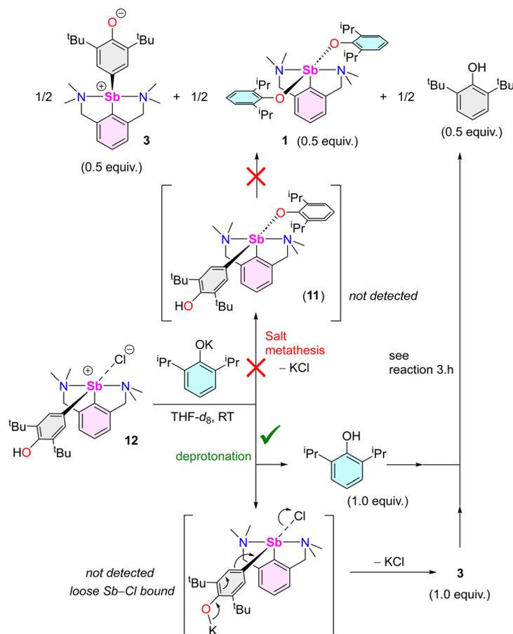
**Scheme 5** Reaction of  $[\{\text{NCN}^{\text{Me}4}\}\text{Sb}(\text{C}_6\text{H}_2\text{-}^t\text{Bu}_2\text{-}3,5\text{-OH-}4)(\text{Cl})]$  (**12**) with  $[\{2,6\text{-}^i\text{Pr}_2\text{-C}_6\text{H}_3\text{O}\}]\text{K}$ , highlighting the two potential mechanistic pathways.
