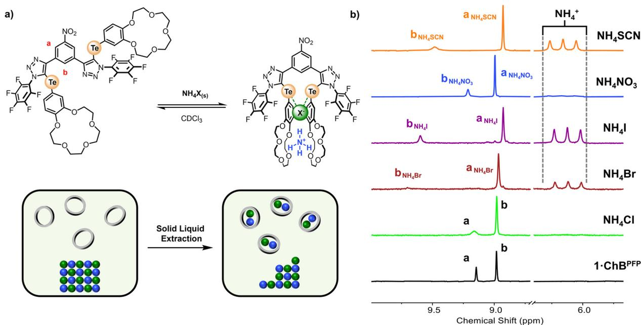
**Fig. 5** (a) Representative SLE equilibrium of ammonium salt ( $\text{NH}_4\text{X}$ ) by  $1\text{-ChB}^{\text{PFP}}$  and cartoon representation of the SLE process (b) Pre and post-SLE  $^1\text{H}$  NMR spectra ( $\text{CDCl}_3$ , 500 MHz, 298 K), with various ammonium salts.
