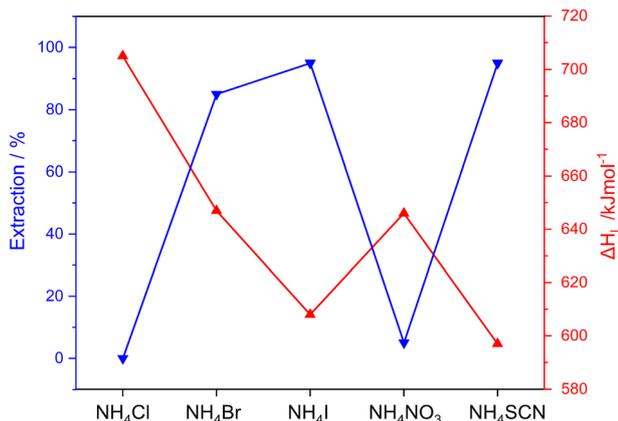
Fig. 6 Plot showing extraction efficiency (blue) and lattice energy  $\Delta H_L$  (red) versus  $\text{NH}_4\text{X}$  ( $\text{X} = \text{Cl}, \text{Br}, \text{I}, \text{NO}_3$ ).
