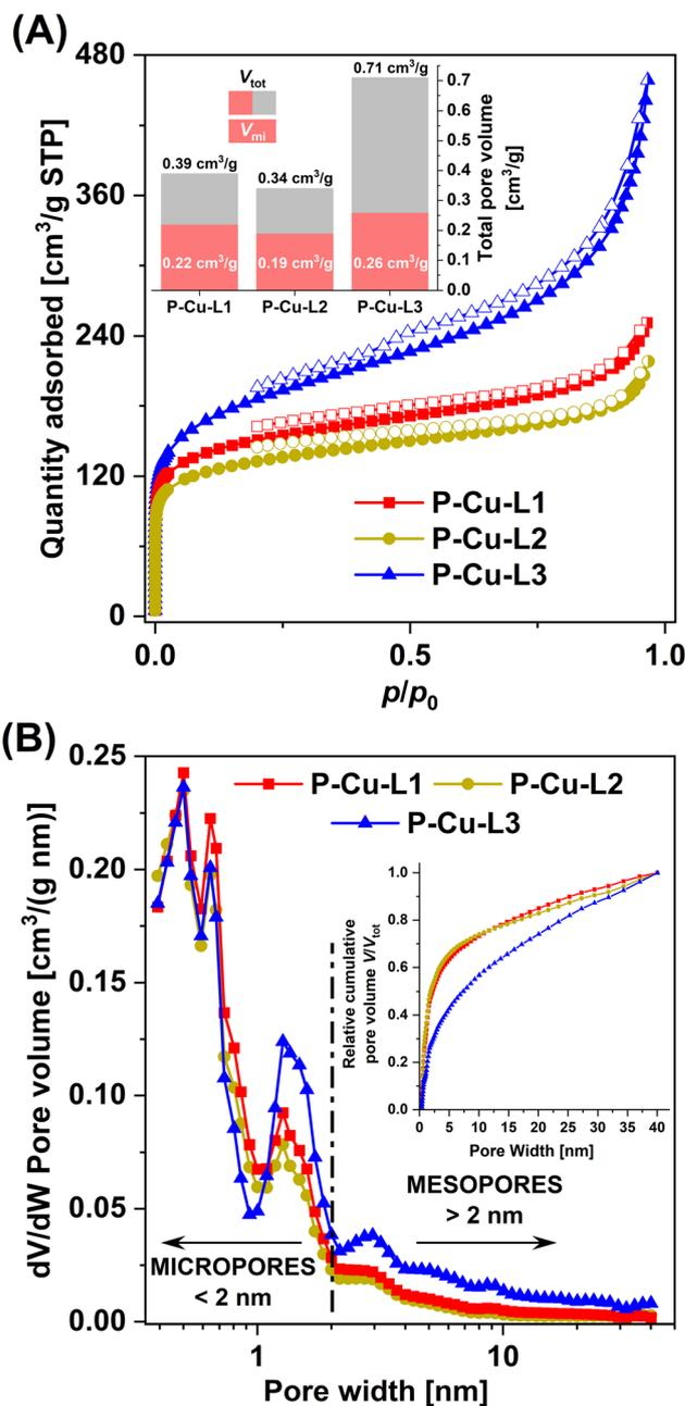
Fig. 7 (A) N<sub>2</sub> adsorption (full symbols) and desorption (empty symbols) isotherms with pore volumes of micropores,  $V_{mi}$ , and total pore volumes,  $V_{tot}$ , for **P-Cu-L1**, **P-Cu-L2** and **P-Cu-L3**. (B) N<sub>2</sub>-DFT calculated pore size distributions with relative cumulative pore volume,  $V/V_{tot}$ , for **P-Cu-L1**, **P-Cu-L2** and **P-Cu-L3**.
