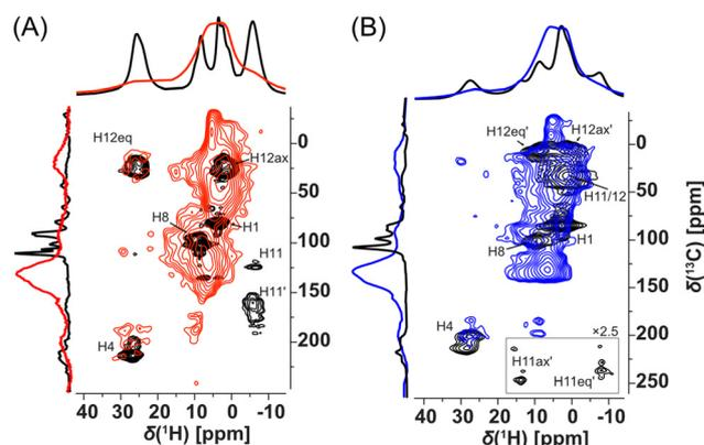
**Fig. 6**  $^1\text{H}$ -detected HSQC-TEDOR spectra (62.5 kHz MAS, 14.09 T) of (A) **Cu-L1** (black) vs. **P-Cu-L1** (red) and (B) **Cu-L3** (black) vs. **P-Cu-L3** (blue). 1D horizontal and vertical traces show direct-excitation spin-echo detected  $^1\text{H}$  and  $^{13}\text{C}$  spectra acquired at 62.5 and 18 kHz, respectively.
