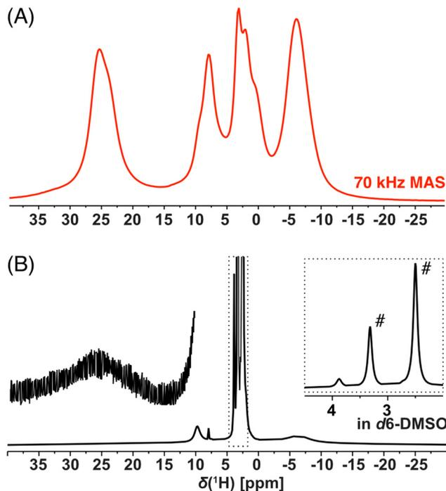
**Fig. 3**  $^1\text{H}$  NMR spectra (14.09 T) of **Cu-L1** acquired by the spin-echo experiment (A) on a solid-state powder sample under 70 kHz MAS conditions and (B) on the  $d_6$ -DMSO solution (# indicate solvent and residual water signals).
