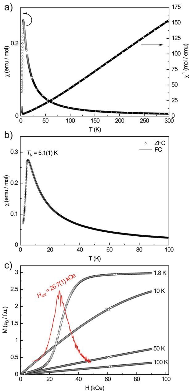
**Fig. 4** Magnetic data of NdAl<sub>5</sub>Pt<sub>3</sub>. (a) Temperature dependence of the magnetic and inverse magnetic susceptibility ( $\chi$  and  $\chi^{-1}$  data) measured with an applied external field of 10 kOe; (b) zero-field-cooled/field-cooled (ZFC/FC) measurements measured with an applied external field of 100 Oe; (c) magnetization isotherms recorded at 1.8, 10, 50 and 100 K, the inflection point is determined by the first derivative of  $dM/dH$ , shown in red.
