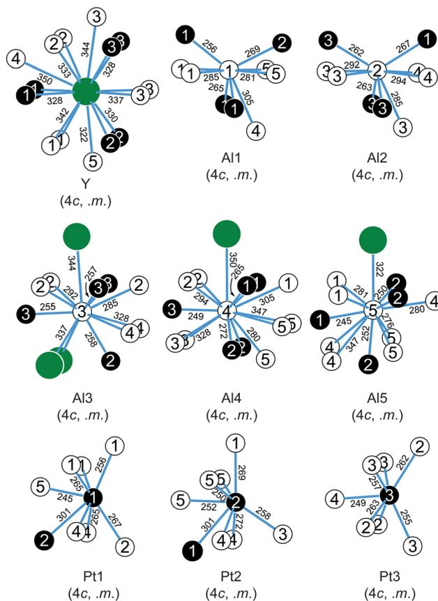
Fig. 3 Coordination environments surrounding the Y, Pt and Al atoms in the structure of  $\text{YAl}_5\text{Pt}_3$ . Sr, Pt and Al atoms are shown as green, white and black circles, respectively. Wyckoff sites, site symmetries and interatomic distances (in pm) are given.
