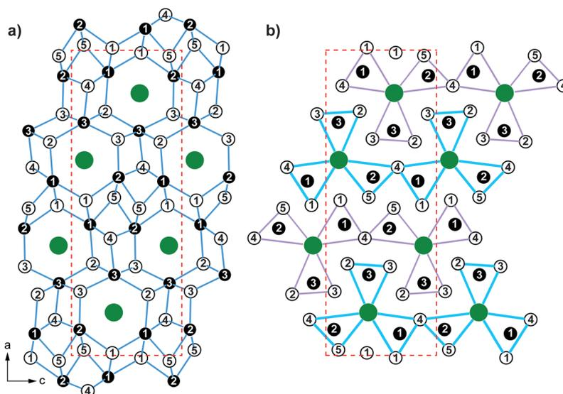
Fig. 2 Unit cell of  $\text{YAl}_5\text{Pt}_3$  as projection along  $[010]$  (a) highlighting the polyanionic  $[\text{Al}_5\text{Pt}_3]^{6-}$  framework (the shortest Al–Pt interactions are emphasized in blue) and (b) using  $\text{XM}_2\text{T}_4$  prisms to illustrate the structure (the interactions forming the prisms are highlighted in blue and purple). Y, Al and Pt atoms are shown in green, white and black circles, respectively.
