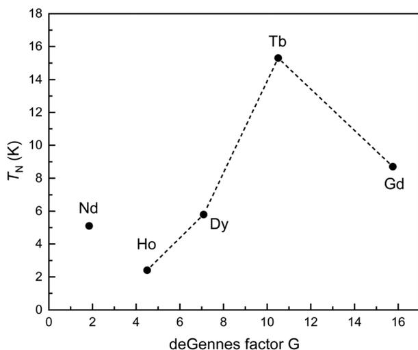
Fig. 5 Plots of the ordering temperatures versus the de Gennes factor  $(g_{\text{J}} - 1)^2 J(J + 1)$  for the  $\text{REAl}_5\text{Pt}_3$  series.
