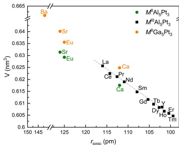
**Fig. 1** Plot of the unit cell volumes (in  $\text{nm}^3$ ) for the  $MAl_5Pt_3$  series ( $M = Ca, Sr, Y, La-Nd, Sm-Er$ ) versus the  $M^{n+}$  radius (in pm). Formally divalent metal atoms are depicted in green, trivalent ones in black, the members of the gallium series are shown in orange.
