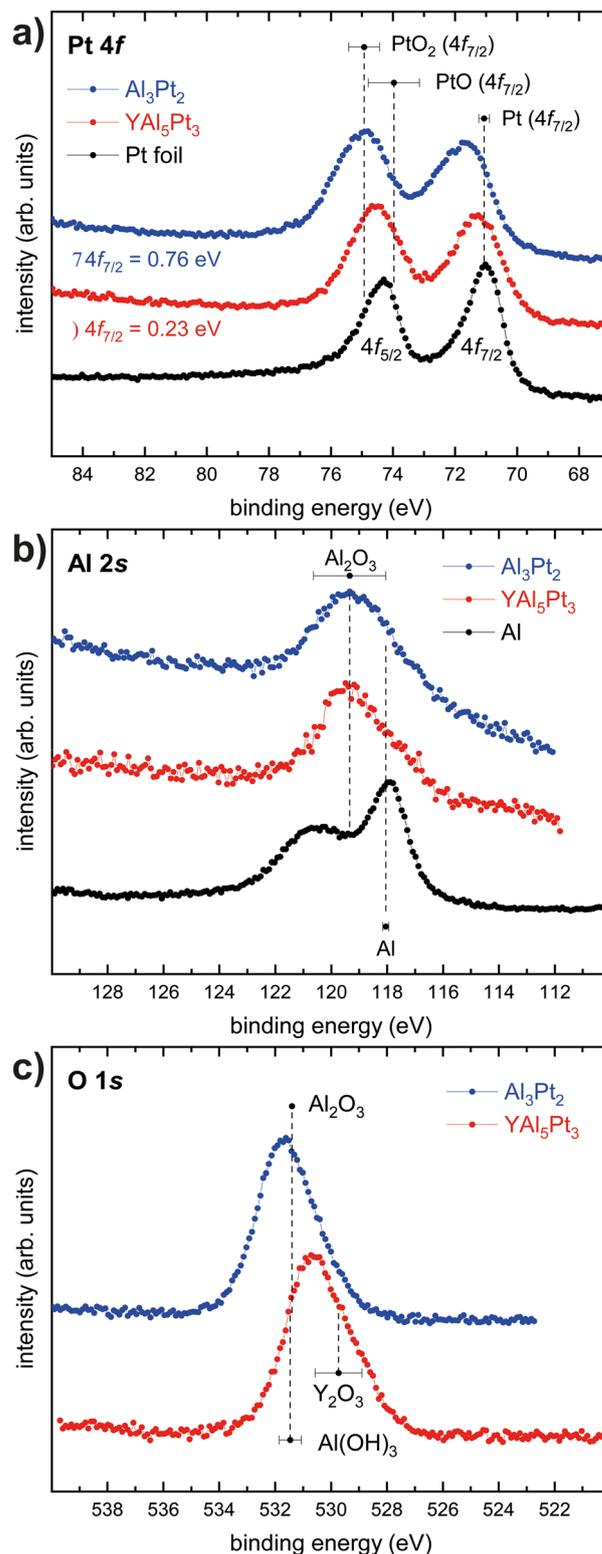
Fig. 7 (a) Pt 4f spectra of  $\text{YAl}_5\text{Pt}_3$  (red) and  $\text{Al}_3\text{Pt}_2$  (blue) and Pt (black); (b) Al 2s spectra of  $\text{YAl}_5\text{Pt}_3$  (red) and  $\text{Al}_3\text{Pt}_2$  (blue) and Al (black); (c) O 1s spectra of  $\text{YAl}_5\text{Pt}_3$  (red) and  $\text{Al}_3\text{Pt}_2$  (blue). Mean values of binding energies and standard deviations are obtained by averaging over all entries in the NIST XPS database for the compounds specified in (a)–(c).<sup>101</sup>
