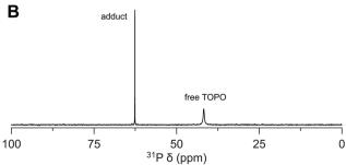
Fig. 6 Interaction of zirconium sec-butoxide with TOPO. (A)  $^{1}$ H NMR of the as-synthesized zirconium( $_{\rm IV}$ ) sec-butoxide to which TOPO is added, and (B)  $^{31}$ P NMR of the mixture in C<sub>6</sub>D<sub>6</sub>.
