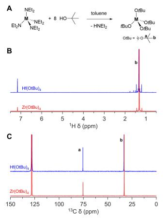
Fig. 4 The synthesis of zirconium(v) and hafnium(v) tert-butoxide complex. (A) General reaction scheme, (B)  $^1$ H NMR, and (C)  $^{13}$ C NMR of zirconium(v) and hafnium(v) tert-butoxide complex in  $C_6D_6$ .
