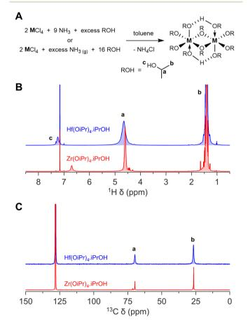
**Fig. 1** The synthesis of zirconium(IV) and hafnium(IV) isopropoxide isopropanol complex. (A) General reaction scheme of both the method making use of ammonia stock solution in isopropanol, and gaseous ammonia, (B)  $^1$ H NMR, and (C)  $^{13}$ C NMR of zirconium(IV) and hafnium(IV) isopropoxide isopropanol complex in  $C_6D_6$ .
