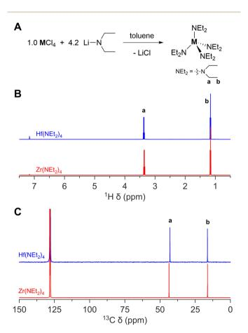
Fig. 3 The synthesis of zirconium( $_{\rm IV}$ ) and hafnium( $_{\rm IV}$ ) diethylamido complex. (A) General reaction scheme, (B)  $^{1}$ H NMR, and (C)  $^{13}$ C NMR of zirconium( $_{\rm IV}$ ) and hafnium( $_{\rm IV}$ ) diethylamido complex in C<sub>6</sub>D<sub>6</sub>.
