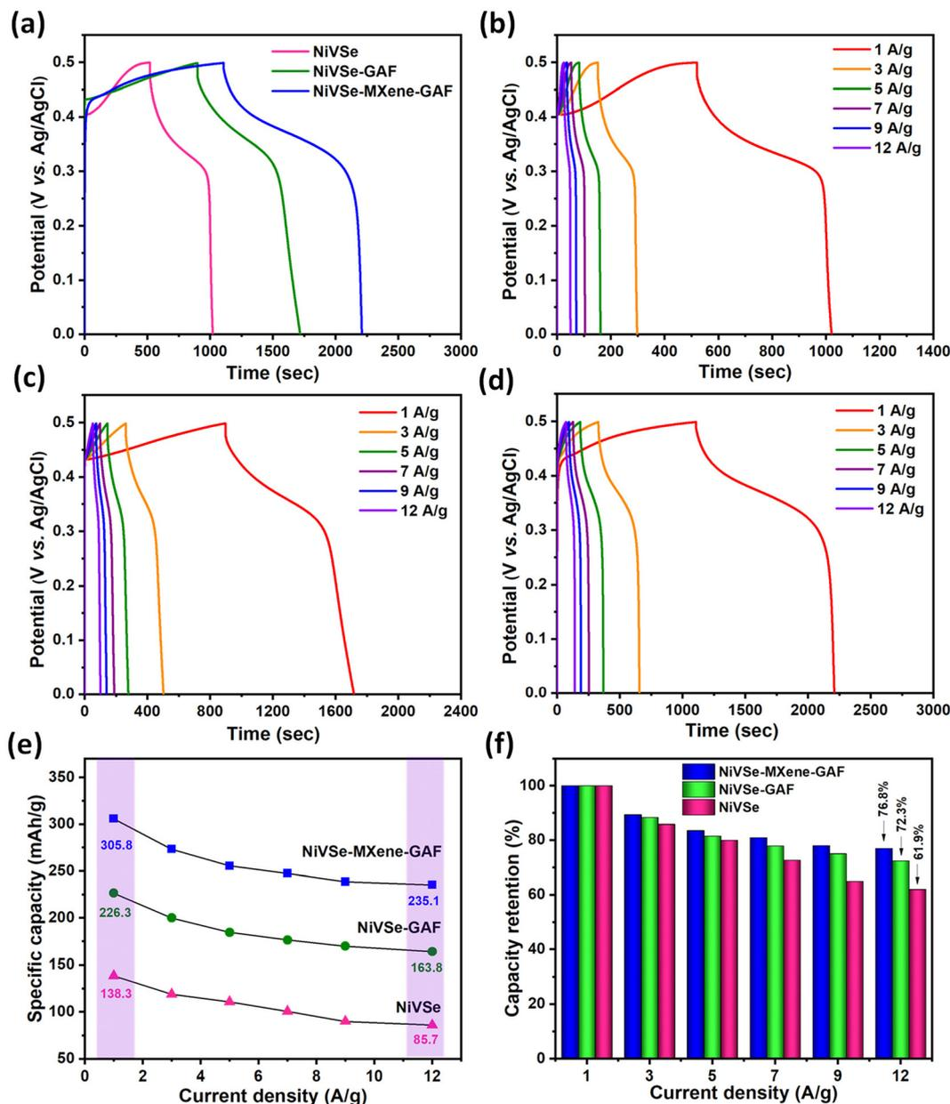
**Fig. 9** (a) GCD plots of NiVSe, NiVSe-GAF, and NiVSe-MXene-GAF at a current density of 1 A g<sup>-1</sup>; GCD plots of (b) NiVSe, (c) NiVSe-GAF, and (d) NiVSe-MXene-GAF at various current densities (1–12 A g<sup>-1</sup>), (e) trend in specific capacity vs. current density for NiVSe, NiVSe-GAF, and NiVSe-MXene-GAF, and (f) capacity retention of NiVSe, NiVSe-GAF, and NiVSe-MXene-GAF with an increase in the current density.
