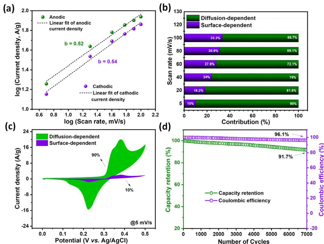
**Fig. 10** (a) Power law plot for NiVSe–MXene–GAF, (b) percentage of diffusion and surface distribution at various scan rates (5–100  $\text{mV s}^{-1}$ ), (c) deconvoluted current density for diffusion and surface contribution at 5  $\text{mV s}^{-1}$ , (d) cycling performance of NiVSe–MXene–GAF for 7000 GCD cycles.
