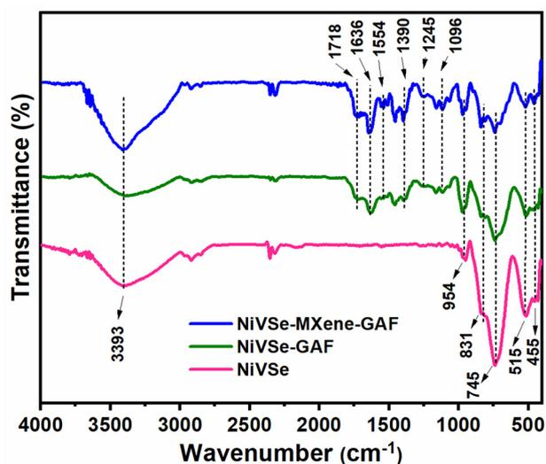
Fig. 5 FT-IR spectra of NiVSe, NiVSe-GAF and NiVSe-MXene-GAF.
