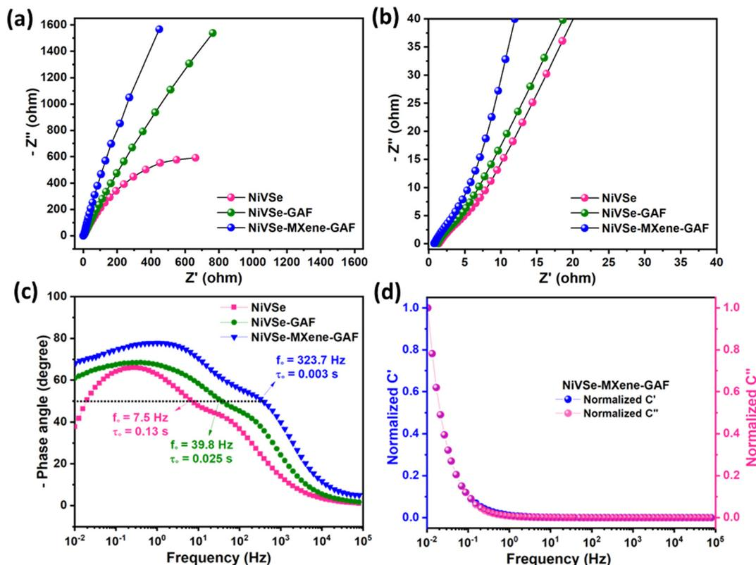
**Fig. 11** EIS measurements: (a) Nyquist plots for NiVSe, NiVSe-GAF, and NiVSe-MXene-GAF, (b) magnified high-frequency region of Nyquist plots (c) Bode plots for NiVSe, NiVSe-GAF, and NiVSe-MXene-GAF, and (d) normalized real ( $C'$ ) and imaginary ( $C''$ ) capacitance vs. applied frequency.
