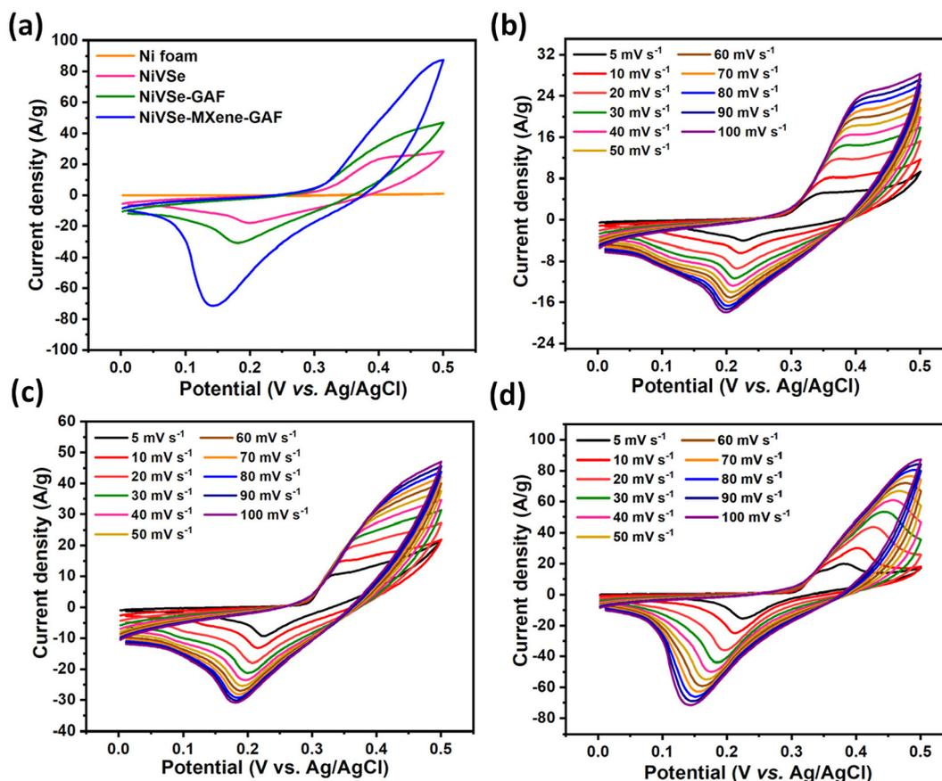
Fig. 8 (a) CV plots of Ni foam, NiVSe, NiVSe-GAF, and NiVSe-MXene-GAF at a scan rate of  $100 \text{ mV s}^{-1}$ ; CV plots of (b) NiVSe (c) NiVSe-GAF, and (d) NiVSe-MXene-GAF at various scan rates ( $5\text{--}100 \text{ mV s}^{-1}$ ).
