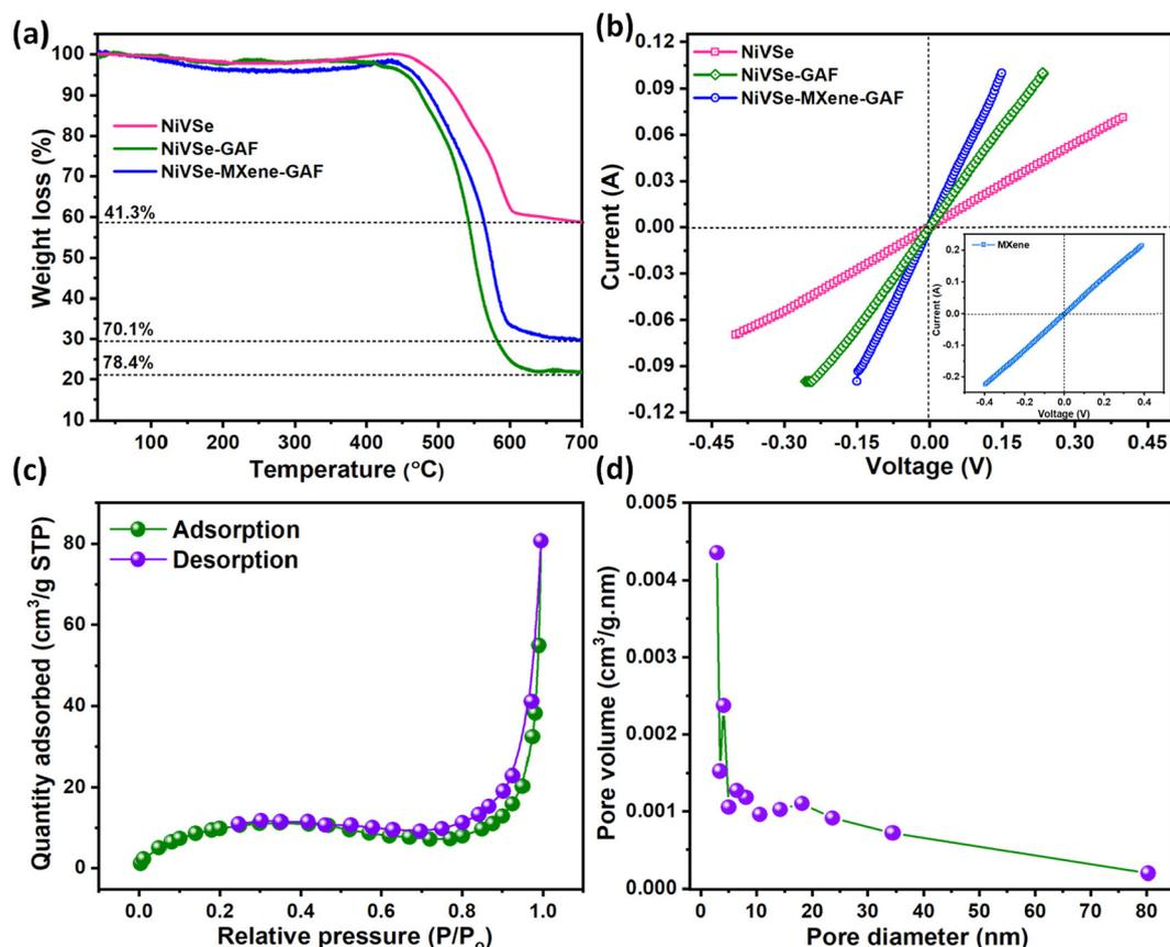
Fig. 7 (a) TGA curves of NiVSe, NiVSe-GAF, and NiVSe-MXene-GAF, (b)  $I$ - $V$  plots of NiVSe, NiVSe-GAF, and NiVSe-MXene-GAF; inset shows the  $I$ - $V$  plot for pure MXene, (c)  $N_2$  adsorption-desorption isotherms for NiVSe-MXene-GAF, and (d) the BJH desorption pore size distribution plot for NiVSe-MXene-GAF.
