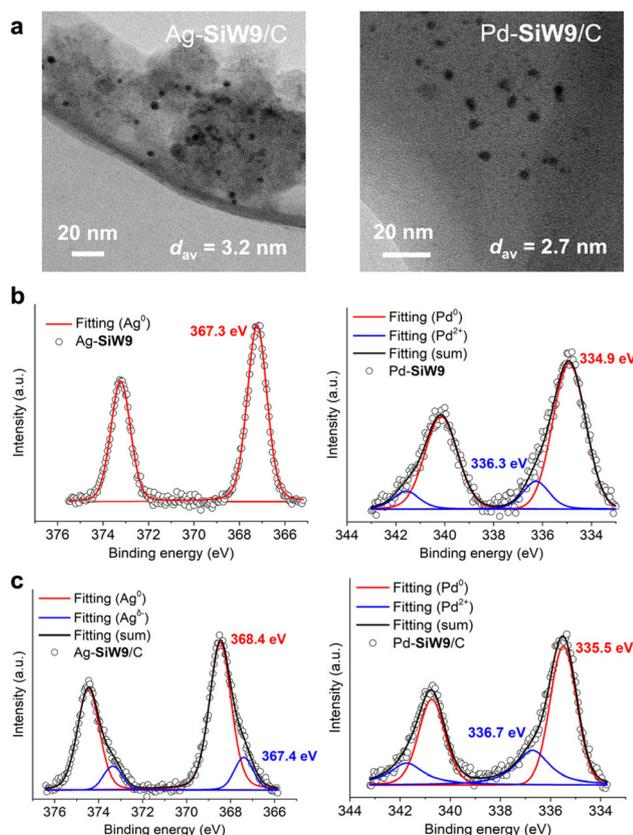
**Fig. 4** (a) TEM images of carbon-supported SiW9-modified Ag and Pd nanoparticles (Ag-SiW9/C and Pd-SiW9/C, respectively). (b and c) XPS spectra of SiW9-modified Ag and Pd nanoparticles: (b) before immobilization (Ag-SiW9 and Pd-SiW9) and (c) after immobilization on carbon supports (Ag-SiW9/C and Pd-SiW9/C).
