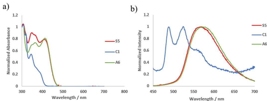
**Fig. 1** (a) Normalized UV-Vis absorption spectra of **S5**, **C1**, and **A6** in degassed DMSO solution ( $10^{-5}$  M); (b) normalized emission spectra of **S5**, **C1**, and **A6** in degassed DMSO solution ( $10^{-5}$  M).
