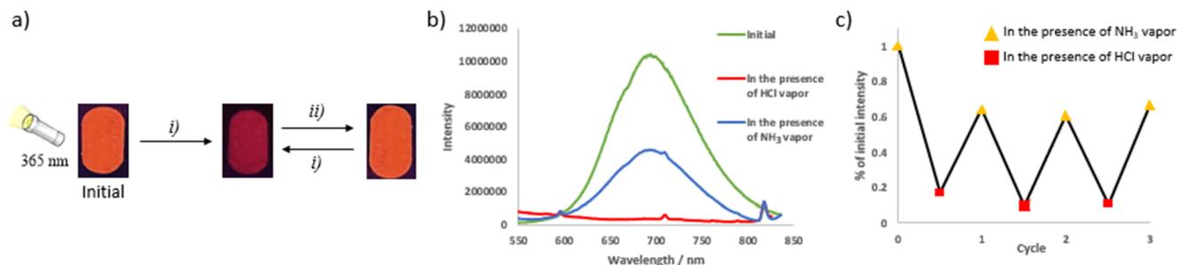
**Fig. 6** (a) Response of **S5** to acids in the solid state (KBr powder with 1% wt of soft salt). Pictures were taken in the dark upon irradiation with a handheld UV lamp ( $\lambda_{\text{em}} = 365 \text{ nm}$ ). Conditions: (i) HCl vapors (ii)  $\text{NH}_3$  vapors; (b) PL spectra of **S5** in the initial state and in presence of HCl/ $\text{NH}_3$  vapors; (c) percentage variation in initial emission intensity measured after 3 repeated exposure cycles to HCl/ $\text{NH}_3$  vapors.
