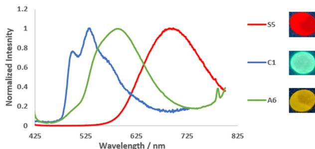
Fig. 3 Left: PL spectra in the solid state of **S5**, **C1**, and **A6** at 298 K. Right: Pictures of KBr pellets of **S5**, **C1**, and **A6** in the dark upon irradiation with a handheld UV lamp ( $\lambda_{\text{em}} = 365$  nm).
