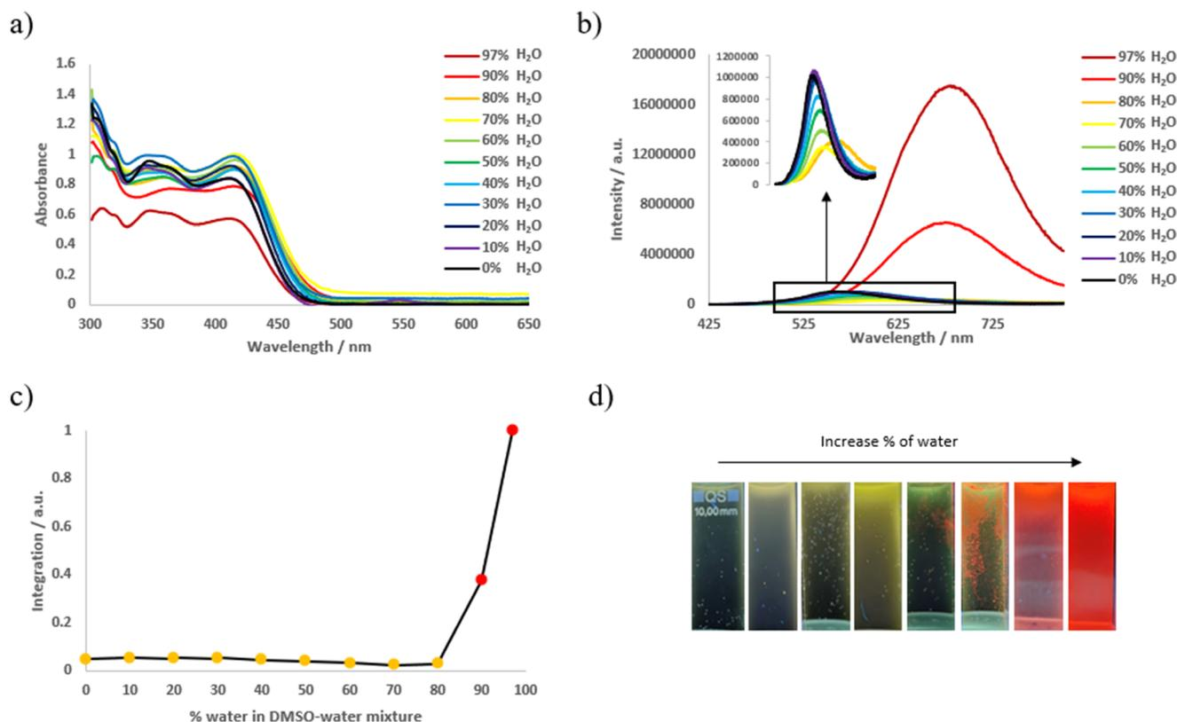
**Fig. 2** (a) UV-Vis absorption spectra of **S5** in DMSO–water mixtures ( $10^{-3}$  M) with different water ratio; (b) emission spectra of **S5** in DMSO–water mixtures ( $10^{-3}$  M) with different water ratio; (c) integration of emission band vs. percentage of water in DMSO/water mixtures; (d) pictures of **S5** solutions in DMSO/water mixtures with various percentages of water taken in the dark upon irradiation with a handheld UV lamp ( $\lambda_{\text{em}} = 254$  nm).
