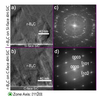
Fig. 2 Cross-section TEM micrographs and corresponding FFT patterns, showing  $r-B_4C$  film-substrate regions from Si-face (a and c) and C-face (b and d) grown films on 4H-SiC. In both cases, the 4H-SiC substrates were aligned along the (11 $\bar{2}$ 0) zone axis.
