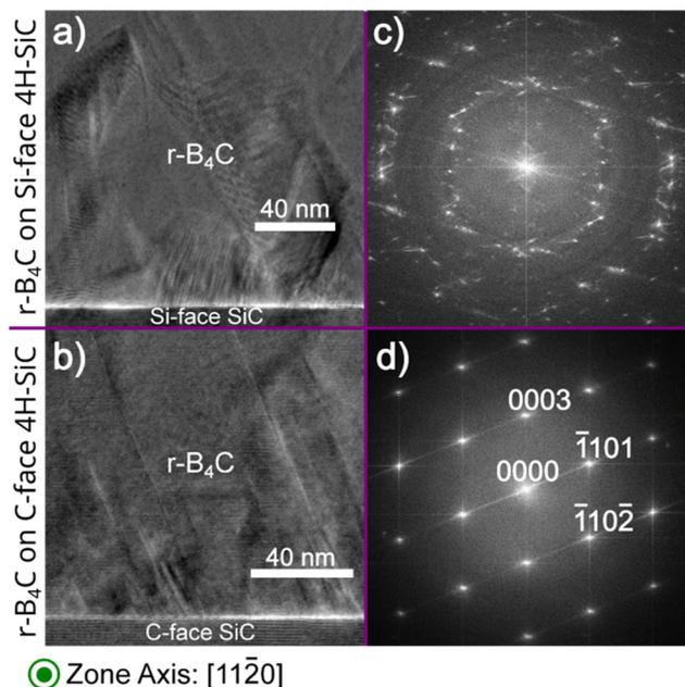
**Fig. 2** Cross-section TEM micrographs and corresponding FFT patterns, showing  $r\text{-B}_4\text{C}$  film-substrate regions from Si-face (a and c) and C-face (b and d) grown films on 4H-SiC. In both cases, the 4H-SiC substrates were aligned along the  $(11\bar{2}0)$  zone axis.
