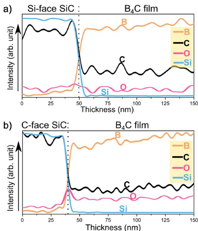
**Fig. 6** EDX depth profiles across the film/substrate interface for r-B<sub>4</sub>C grown on the Si-face (a) and C-face (b) of 4H-SiC. The intensities have been shifted along the y-axis to show a better reflection of the elemental distribution.
