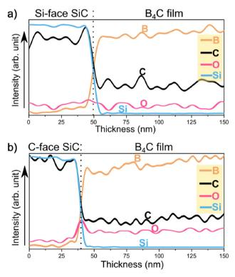
Fig. 6 EDX depth profiles across the film/substrate interface for  $r-B_4C$  grown on the Si-face (a) and C-face (b) of 4H-SiC. The intensities have been shifted along the *y*-axis to show a better reflection of the elemental distribution.
