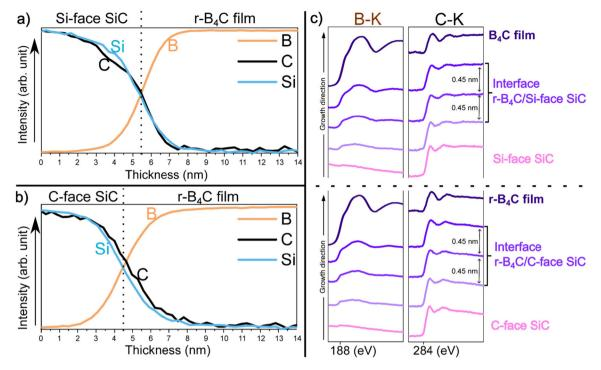
Fig. 5 Elemental distribution profiles across the film/substrate interface for  $r-B_4C$  grown on the Si-face (a) and C-face (b) of 4H-SiC. Stacked B-K and C-K edge EELS spectra are also shown for the respective substrates in (c). We note that the C signal for  $r-B_4C$  film in both (a) and (b) is not zero/noise level but, instead, the lowest in this measured range *i.e.* in the  $B_4C$  film. This is a consequence of the normalization of the EELS signal in the measured thickness range shown.
