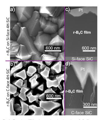
Fig. 1 Top-view SEM micrographs showing the r-B<sub>4</sub>C film morphologies grown on the Si-face (a) and the C-face (b) of 4H-SiC. Cross-section STEM-HAADF micrographs show corresponding film microstructures on the Si-face (c) and C-face (d) of 4H-SiC with voids indicated by dotted lines.
