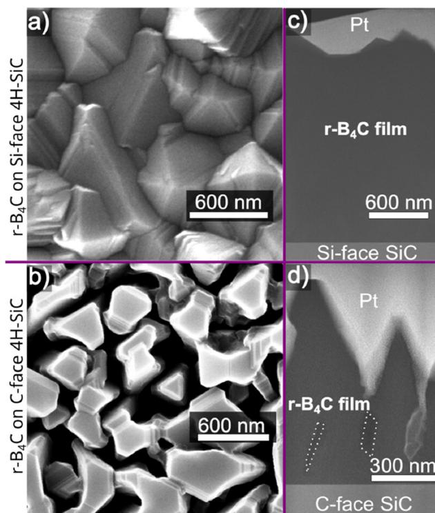
**Fig. 1** Top-view SEM micrographs showing the  $r\text{-B}_4\text{C}$  film morphologies grown on the Si-face (a) and the C-face (b) of 4H-SiC. Cross-section STEM-HAADF micrographs show corresponding film microstructures on the Si-face (c) and C-face (d) of 4H-SiC with voids indicated by dotted lines.
