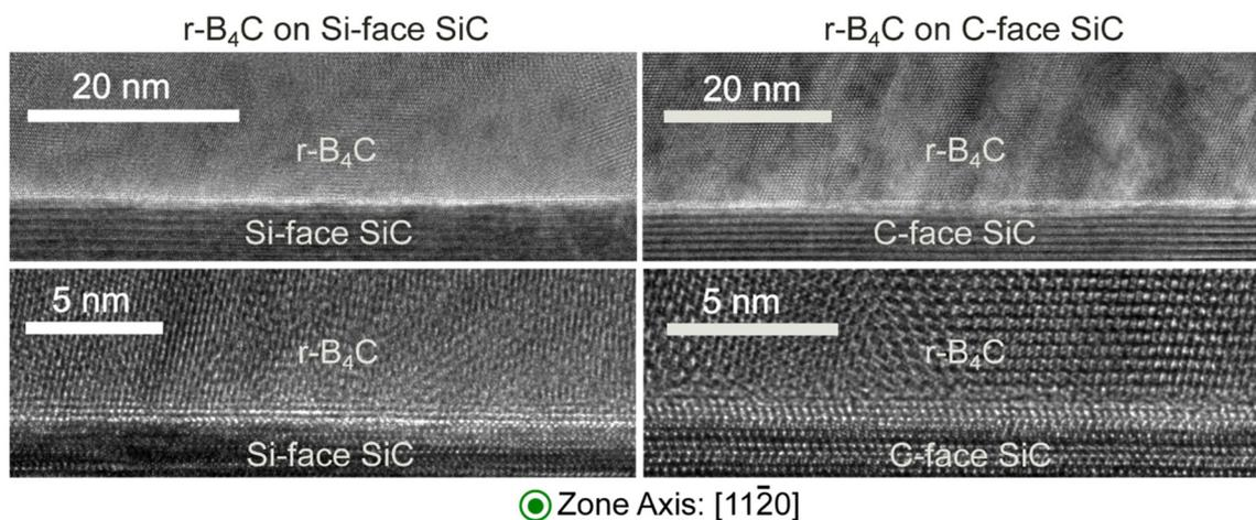
**Fig. 4** Cross-section HRTEM micrographs of the film/substrate interface viewed along the  $(11\bar{2}0)$  zone axis at three different magnification values. No apparent differences in substrate roughness are observed between the two substrates. No indication of additional interlayer formation is observed between the film and the substrate for either sample.
