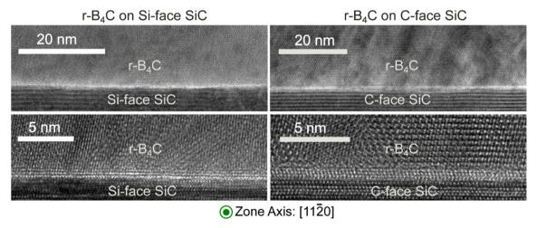
Fig. 4 Cross-section HRTEM micrographs of the film/substrate interface viewed along the (1120) zone axis at three different magnification values. No apparent differences in substrate roughness are observed between the two substrates. No indication of additional interlayer formation is observed between the film and the substrate for either sample.
