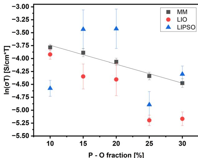
Fig. 5 Logarithm of room temperature conductivity values, derived from EIS measurements, plotted against the total P–O fraction for LIPSO, LIO, and mechanical mix (MM) synthesis procedures.
