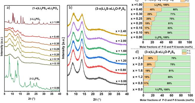
Fig. 2 (a and b) X-ray diffractograms of LIPSO (a) and LIO (b) series. (c and d) Fraction of P-O and P-S bonds in the materials from LIPSO (c) and LIO (d) series, showing the equivalence of both experimental series (a and c taken from Luo 2022).<sup>53</sup>
