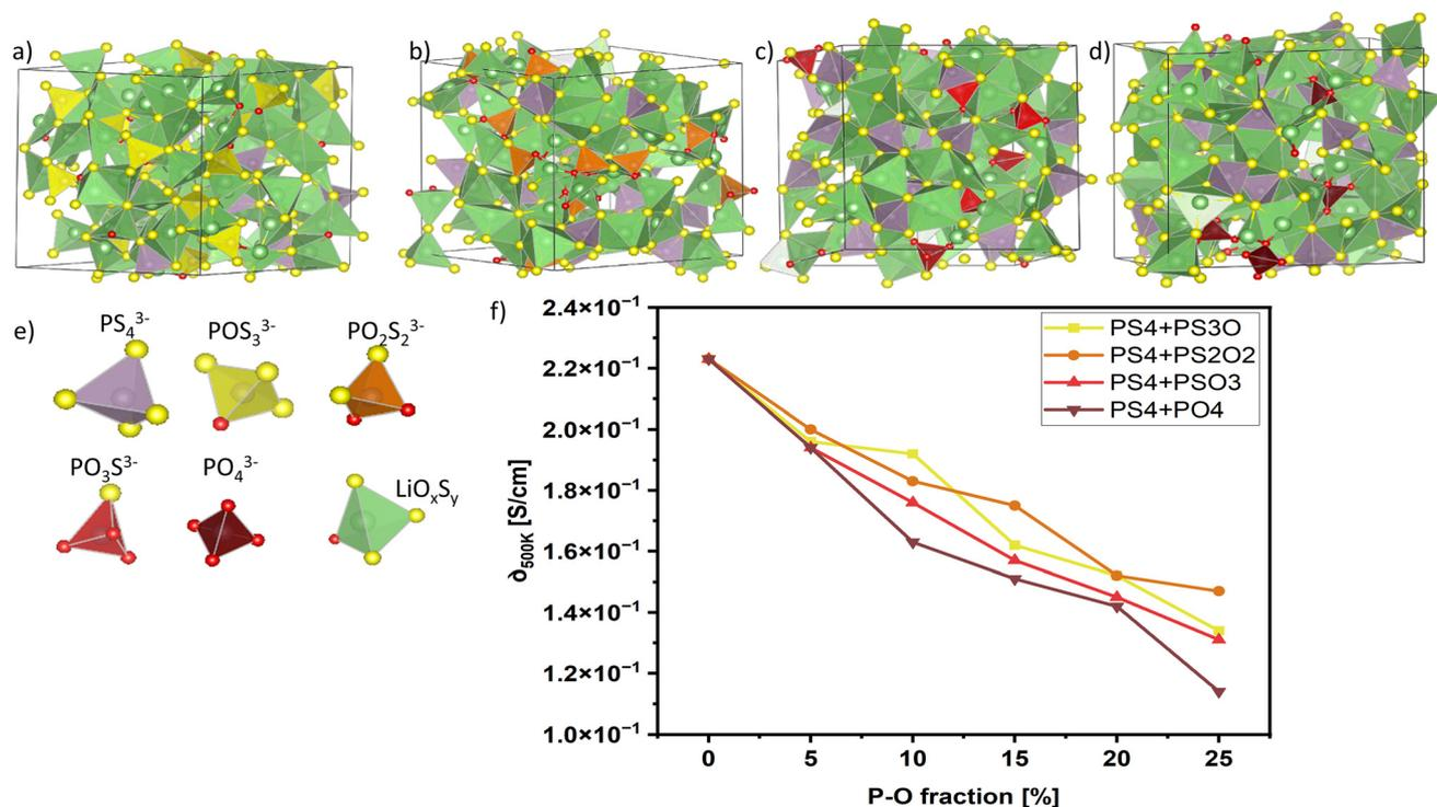
Fig. 8 (a–d) Simulated structures with only  $\text{PS}_4$  and  $\text{POS}_3$  (a),  $\text{PO}_2\text{S}_2$  (b),  $\text{PO}_3\text{S}$  (c),  $\text{PO}_4$  (d) units at 20% P–O fraction. (e) Description of the different polyhedra. (f) Calculated Li-ion conductivities against P–O fraction for the displayed structures.
