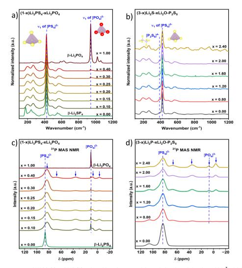
Fig. 4 (a and b) Raman spectra of LIPSO (a) and LIO (b) series with assignment of the main bands and sketches of  $PS_4^{3-}$ ,  $PO_4^{3-}$ , and  $P_2S_6^{4-}$  structural units. (c and d) <sup>31</sup>P MAS NMR spectra of LIPSO (c) and LIO (d), blue arrows pointing to the peaks of mixed [PO<sub>x</sub>S<sub>4-x</sub>]<sup>3-</sup> (a and c taken from Luo 2022).53
