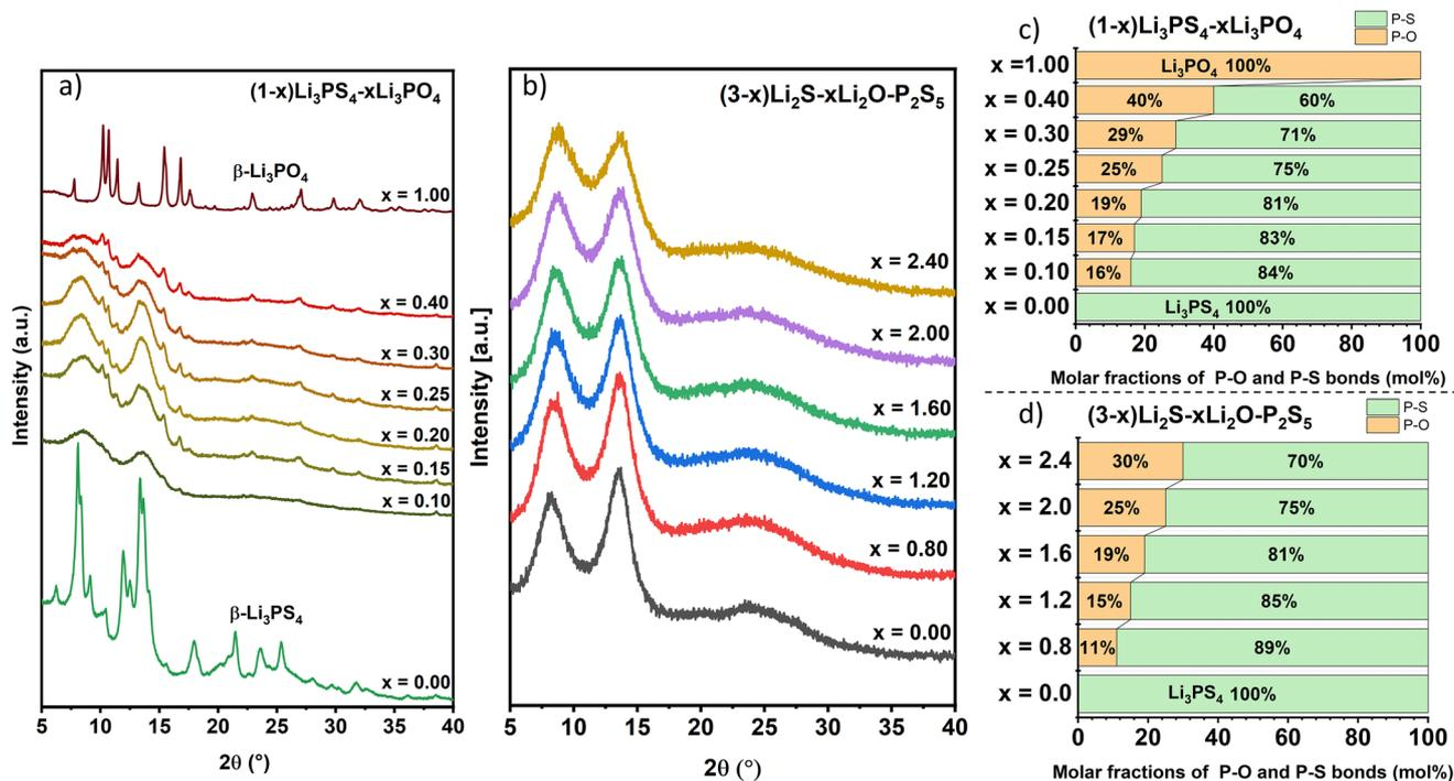
**Fig. 2** (a and b) X-ray diffractograms of LIPSO (a) and LIO (b) series. (c and d) Fraction of P-O and P-S bonds in the materials from LIPSO (c) and LIO (d) series, showing the equivalence of both experimental series (a and c taken from Luo 2022).<sup>53</sup>
