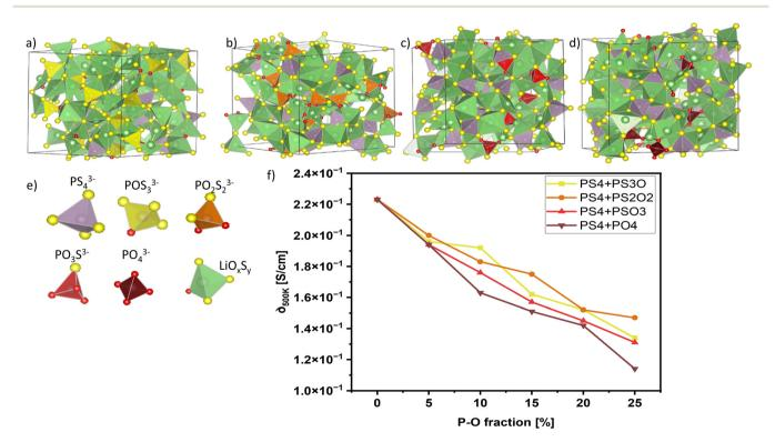
Fig. 8 (a-d) Simulated structures with only PS<sub>4</sub> and POS<sub>3</sub> (a), PO<sub>2</sub>S<sub>2</sub> (b), PO<sub>3</sub>S (c), PO<sub>4</sub> (d) units at 20% P-O fraction. (e) Description of the different polyhedra. (f) Calculated Li-ion conductivities against P-O fraction for the displayed structures.
