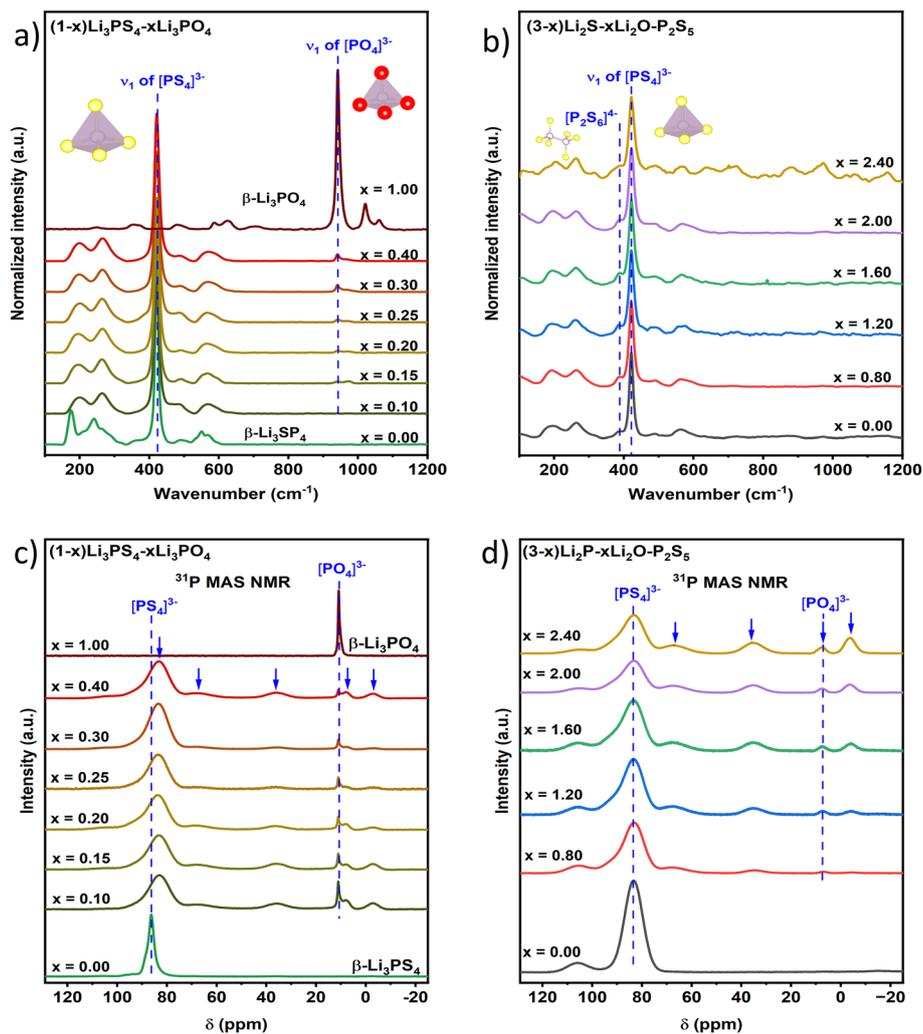
**Fig. 4** (a and b) Raman spectra of LIPSO (a) and LIO (b) series with assignment of the main bands and sketches of  $\text{PS}_4^{3-}$ ,  $\text{PO}_4^{3-}$ , and  $\text{P}_2\text{S}_6^{4-}$  structural units. (c and d)  $^{31}\text{P}$  MAS NMR spectra of LIPSO (c) and LIO (d), blue arrows pointing to the peaks of mixed  $[\text{PO}_x\text{S}_{4-x}]^{3-}$  (a and c taken from Luo 2022).<sup>53</sup>
