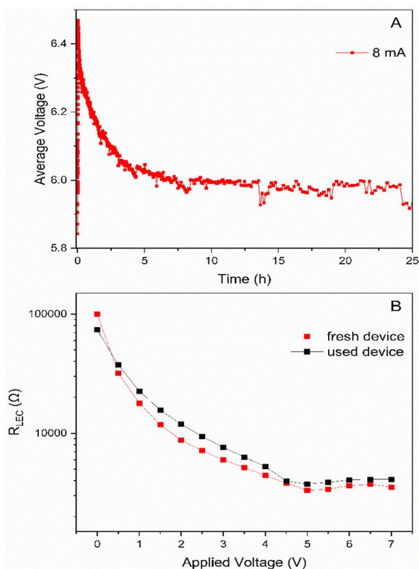
**Fig. 6** (A) Average voltage profile vs. time of [Ag(IPr)(bpy)][PF<sub>6</sub>]-based LECs operating at a pulsed current of 8 mA. (B) LEC resistance vs. applied voltage for fresh and used [Ag(IPr)(bpy)][PF<sub>6</sub>] based LECs – see the legend.
