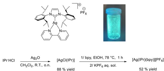
**Fig. 1** The chemical structure, picture of the powder under 305 nm UV lamp irradiation, and synthesis scheme of [Ag(IPr)(bpy)][PF<sub>6</sub>].
