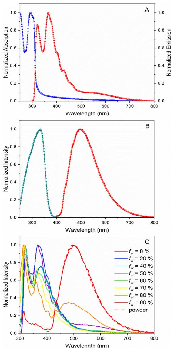
**Fig. 3** (A) UV-Vis absorption (blue) and emission (red) spectra of [Ag(IPr)(bpy)][PF<sub>6</sub>] in THF solution. (B) Emission (red) and excitation (green) spectra of [Ag(IPr)(bpy)][PF<sub>6</sub>] in powder at RT. (C) Emission spectral changes of [Ag(IPr)(bpy)][PF<sub>6</sub>] in volume mixtures of THF : H<sub>2</sub>O – see the legend, highlighting the AIE effect that leads to the same emission band in any aggregated state (powder and solution suspension).
