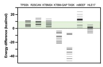
**Fig. 3** High- and low-spin energy differences for the test case with different exchange-correlation functionals. The green energy range indicates the region where the energy difference (below 10 kcal mol<sup>-1</sup>) can be compensated by the entropy in a common spin-crossover compound. TPSSh results were previously published. For the six non-hybrid *meta*-GGA functionals, the same PBE-MB optimized geometry was employed.
